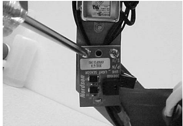
Figure 5-15 Light Detector Board Replacement
