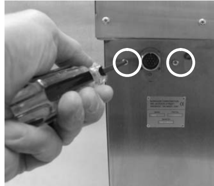
Figure 5 Removing Screws by Unicable
