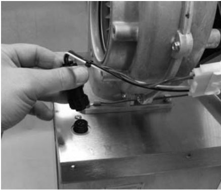
Figure 2 Unplugging Blower Cable
