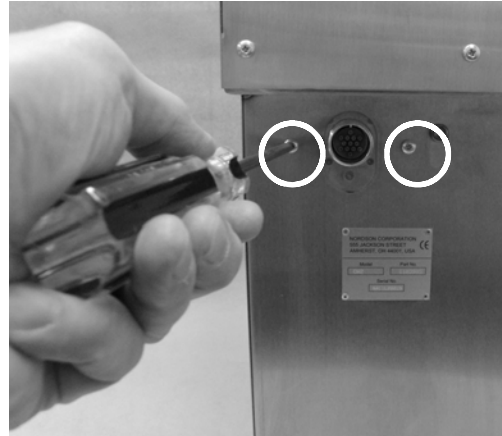
Removing Screws at Unicable Receptacle
