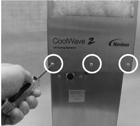
Figure 6-12 Removing Top Blower Cover
