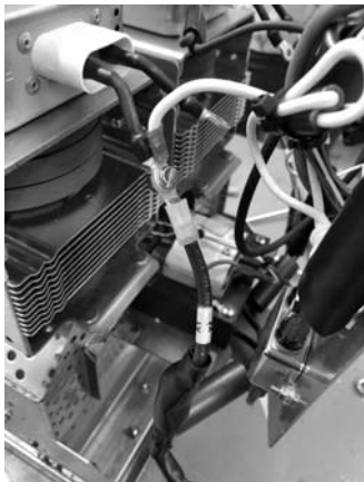
Figure 13 Connecting Ring Terminals on Left Magnetron
