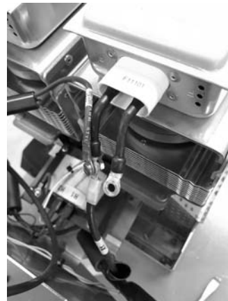
Figure 14 Connecting Ring Terminals on Right Magnetron
