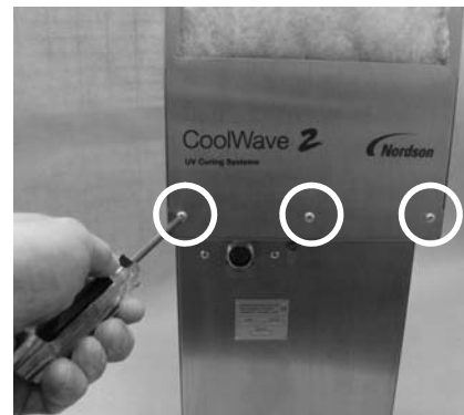
Figure 1 Removing Blower Screws
