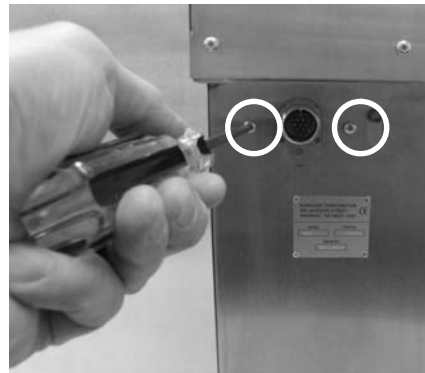
Figure 5 Removing Screws by Unicable
