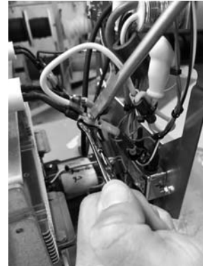
Figure 10 Disconnecting Ring Terminals
