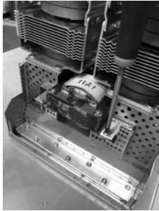
Figure 16 Installing Bracket Screws
