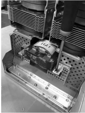
Figure 8 Removing Bracket Screws
