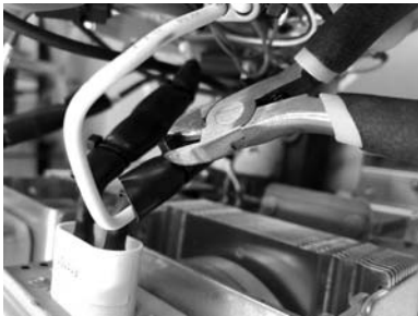
Figure 9 Cutting Cable Ties
