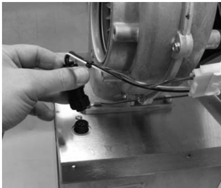
Figure 2 Unplugging Blower Cable
