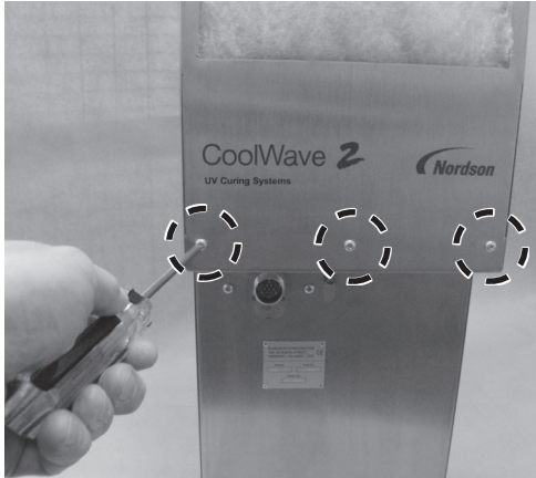
Removing Screws from Top Cover
