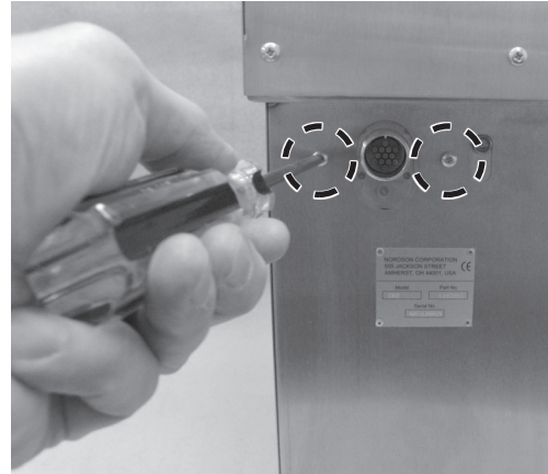
Removing Screws at Unicable Receptacle
