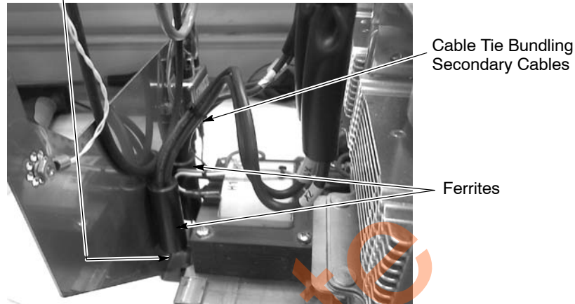
Figure 6-22 Installing Cable Ties on Secondary Cables
