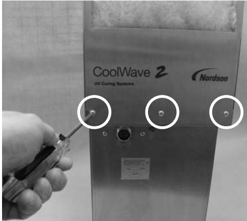
Figure 6-12 Removing Top Blower Cover
