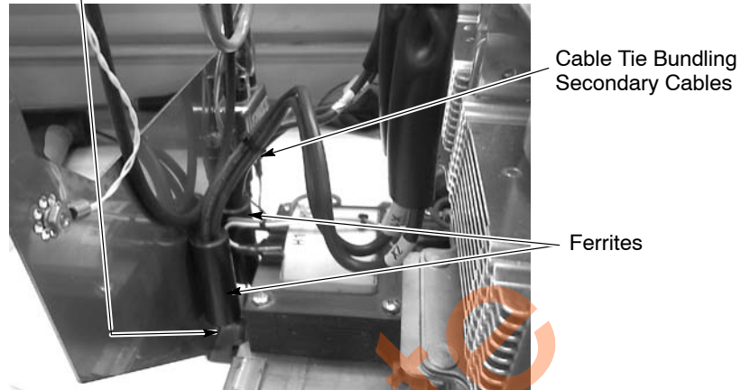
Figure 6-22 Installing Cable Ties on Secondary Cables
