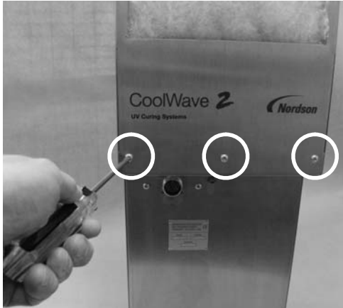
Figure 6-12 Removing Top Blower Cover
