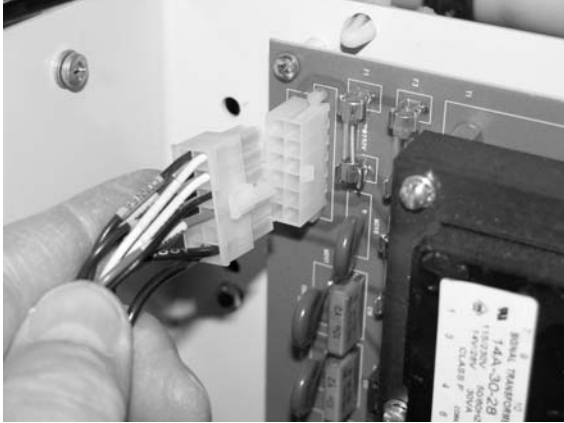
Unclip Power Connector
