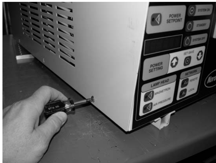
Figure 3 Remove Cover Screws
