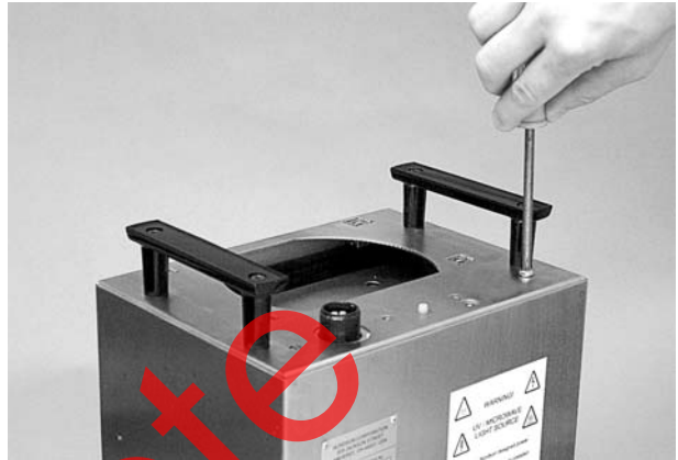
Figure 4-9 Lamphead Cover Removal (Top Four Screws)
