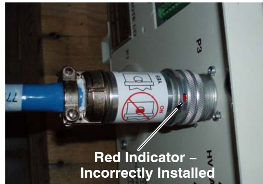
Figure 3-9 Unicable connector partially installed
