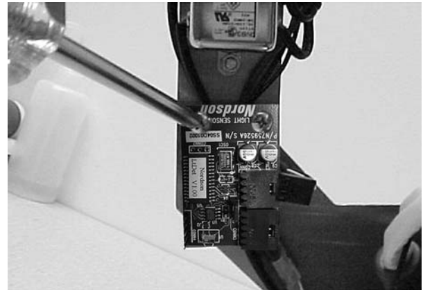
Figure 4-15 Light Detector Board Replacement
