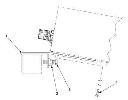
Figure 16 Rail-Mounting Bracket
