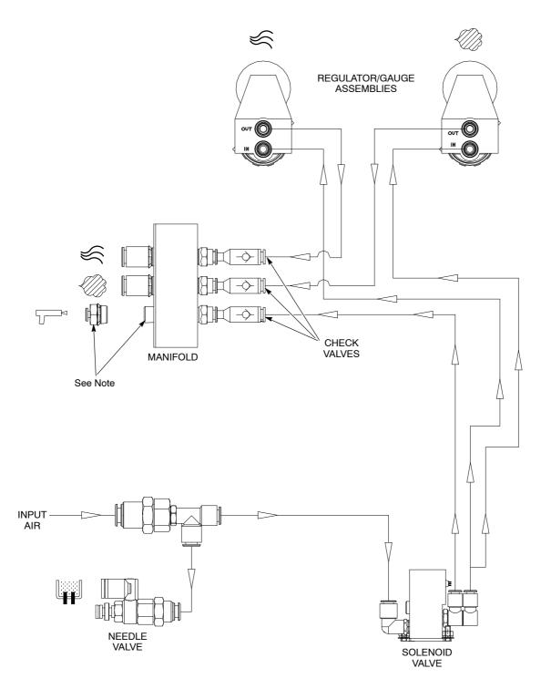
Figure 11 Pneumatic Schematic
