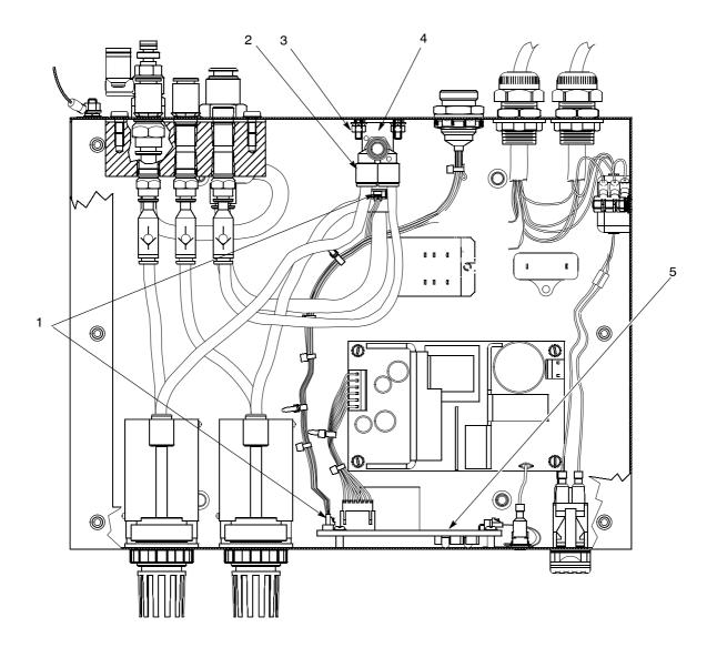
Figure 13 Solenoid Valve Replacement
