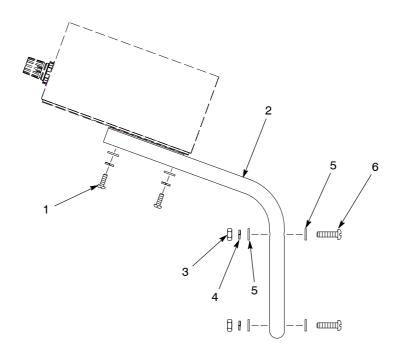
Figure 17 Wall-Mounting Bracket
