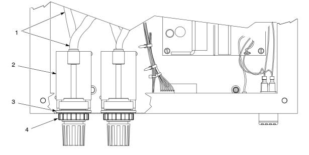
Figure 12 Regulator Assembly Replacement
