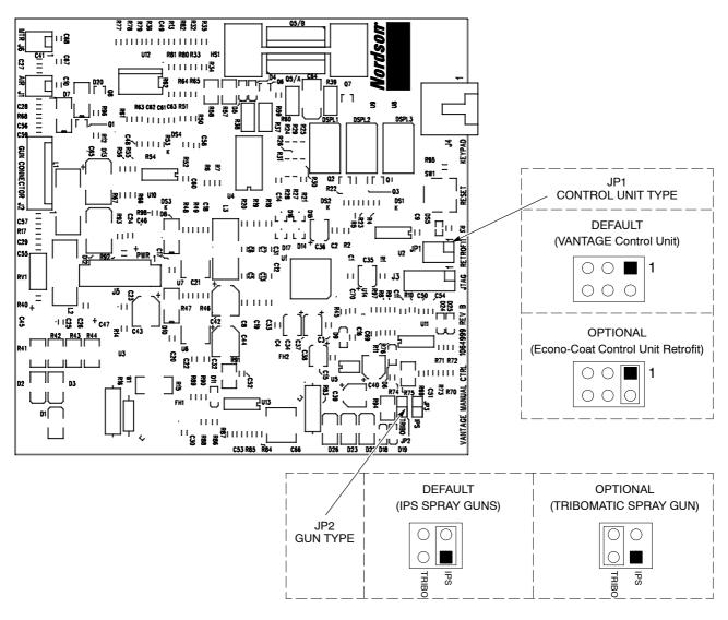
Figure 3 Circuit Board Configuration
