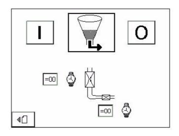
Pressing the "=00" box will take you to the data entry screen, which allow you to set the top pinch valve opening time. This should be set between 10–30 (x100 milliseconds).
