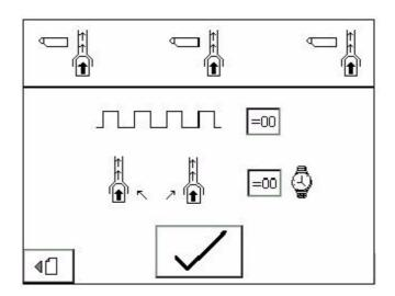
Pressing the "=00" box takes you to the data entry screen, which allows you to set how many pump purges are required.
