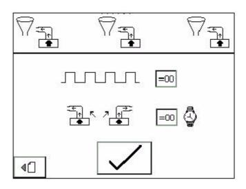
Pressing on the "=00" box takes you to the data entry screen, which allows you to set how many pump purges are required.
