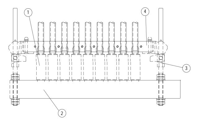
Fig. 7-6 Light/Dark Manifold for Straight Through Pumps
