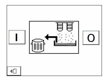
Press this icon to switch on the transfer pump and fluid bed, which empties the rear waste hopper, when fitted.
