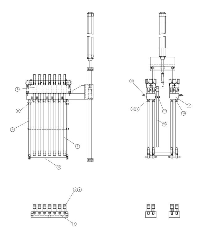
Fig. 7-4 Straight Through 14 Pump Lance Assembly
