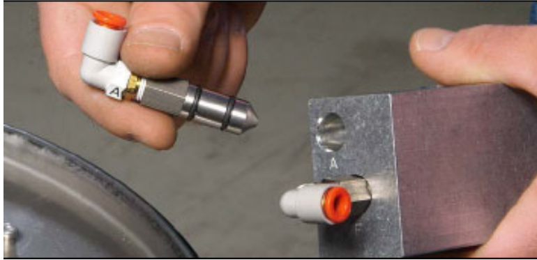
Fig. 5-13 O-rings on the Venturi nozzle
