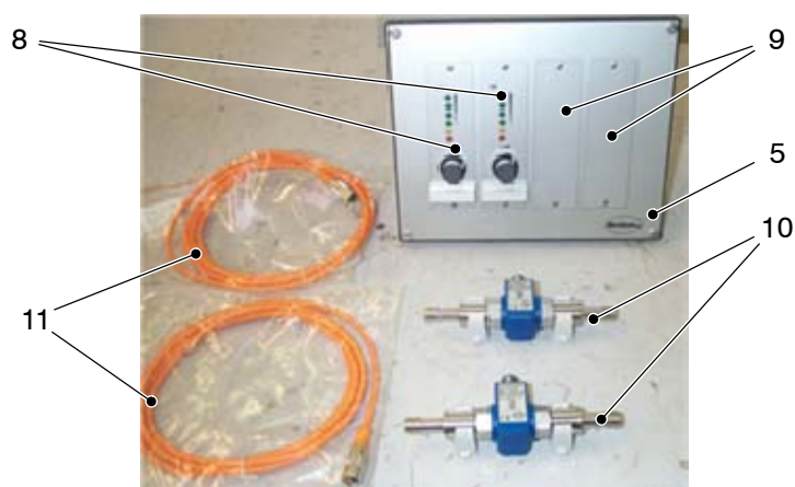
Fig. 2 KIT PFC: Control unit (two channels) w/ sensors and cables
