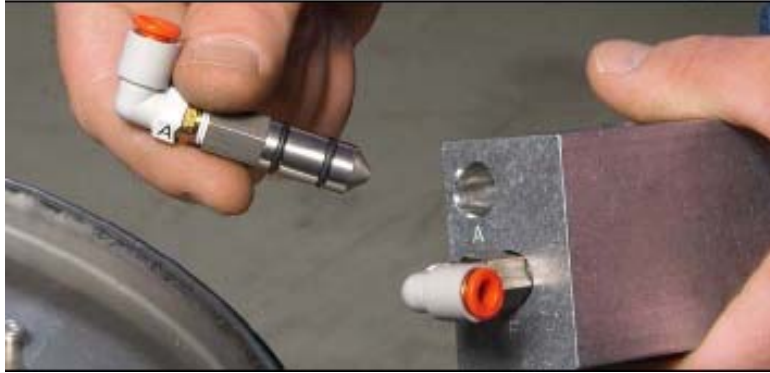
Fig. 5-14 O-rings on the Venturi nozzle
