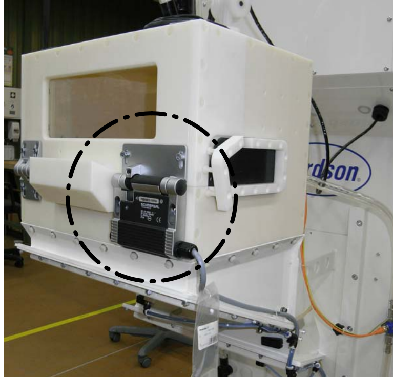
Fig. 10-3 Example of a spray chamber with safety switch
