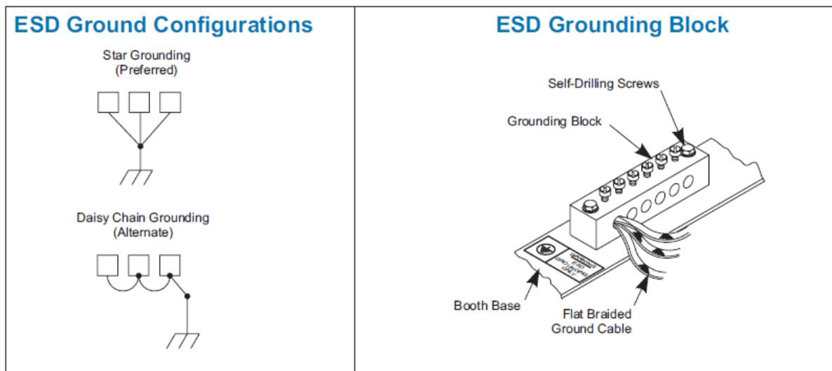
Figure 1 ESD Ground Procedures and Equipment
