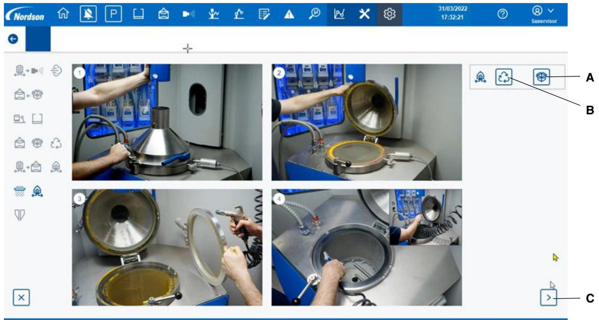
Figure 25 Spectrum HD - Colour Change (Step 7)
