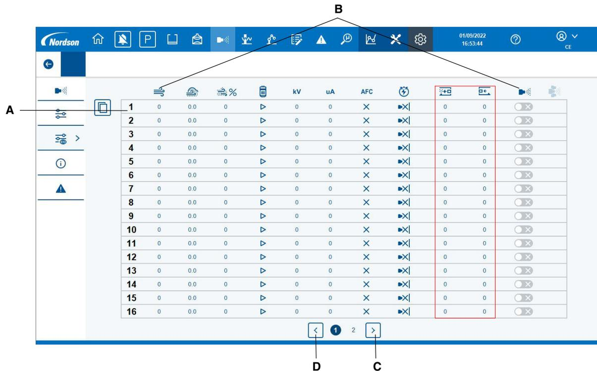
Figure 32 16 Gun Setpoint Control Screen
