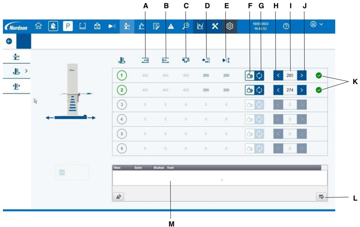
Figure 38 Z-Axis Control Screen
