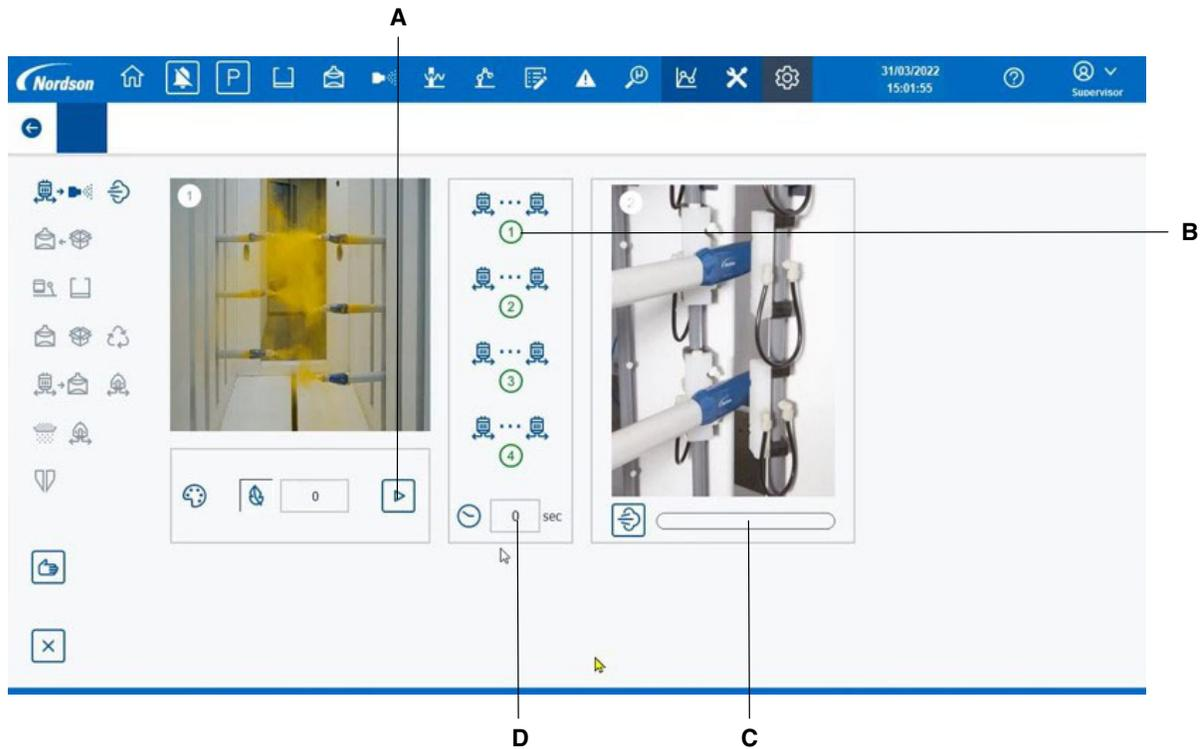
Figure 20 Spectrum HD - Colour Change (Step 2)
