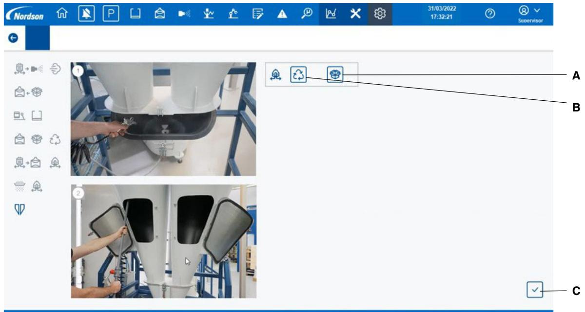
Figure 26 Spectrum HD - Colour Change (Step 8)
