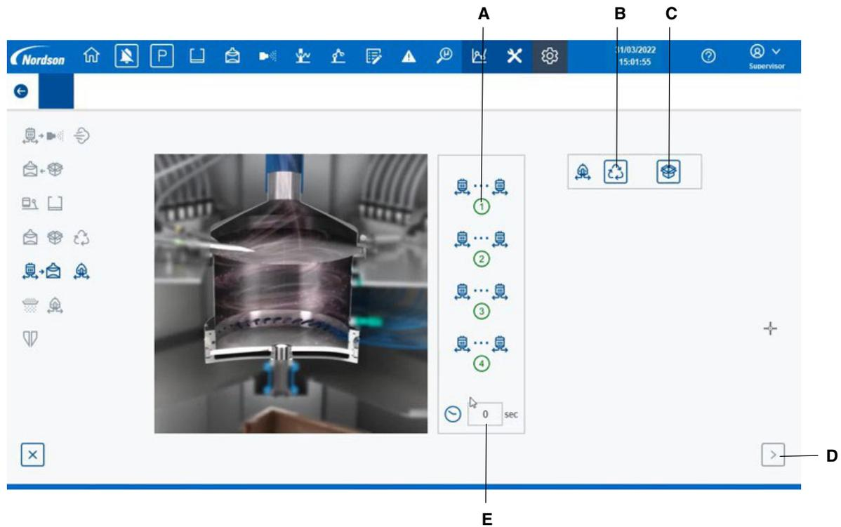
Figure 24 Spectrum HD - Colour Change (Step 6)
