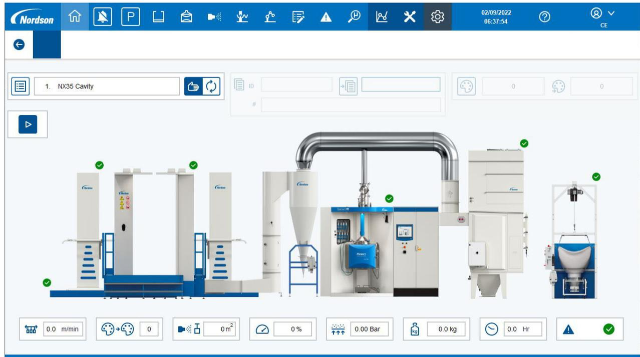
The Nordson PowderPilot™ 4.X is an intuitive control system, with software and hardware specifically designed for automated powder coating systems. It delivers precision digital control for your paint line for easy access to all powder application and booth operating parameters. The touch screen is used for all interactions between the operator and the machine.
