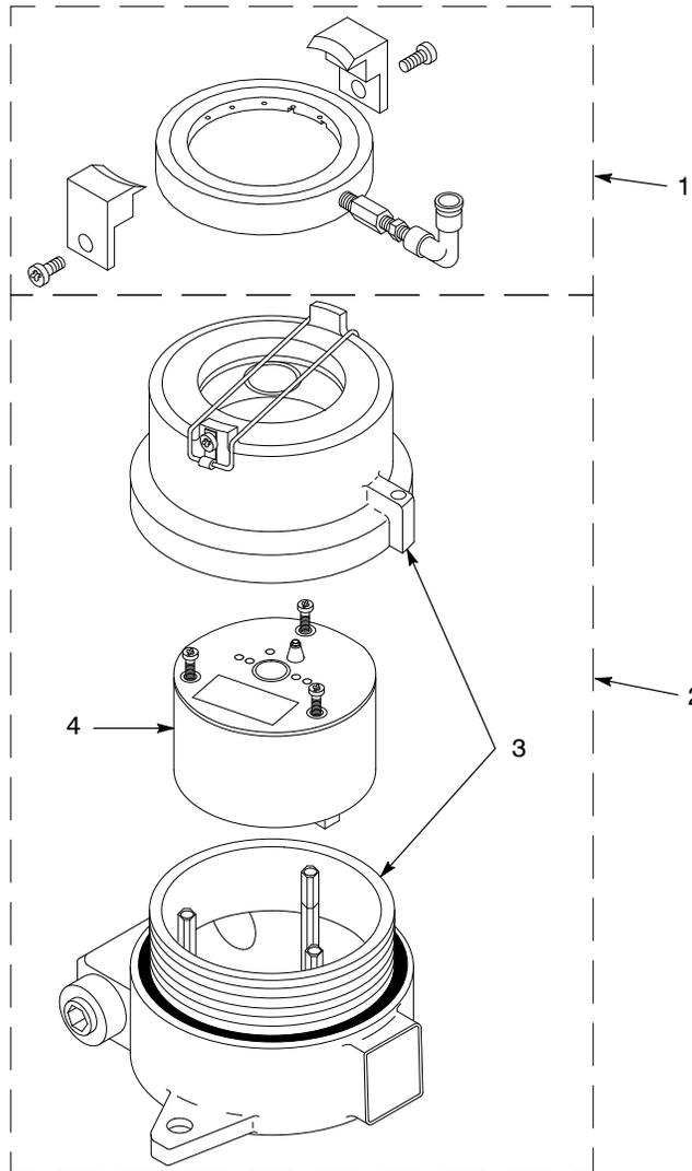
Figure 10 Detector Head Parts
