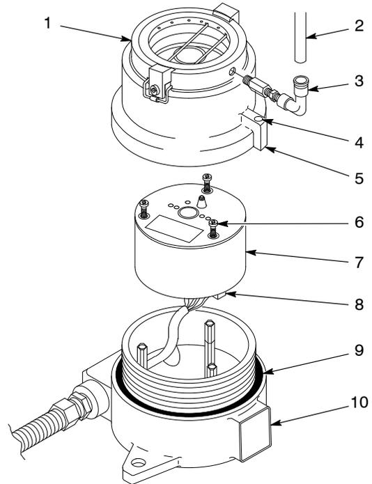
Figure 9 Detector Head Electrical Connections
