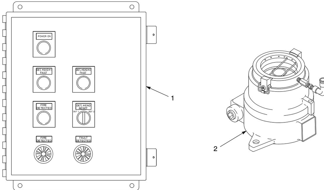
Figure 1 FS10-R30 Flame Detector Components
