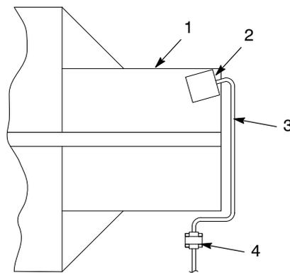
Figure 4 Detector Head Pneumatic Connections
