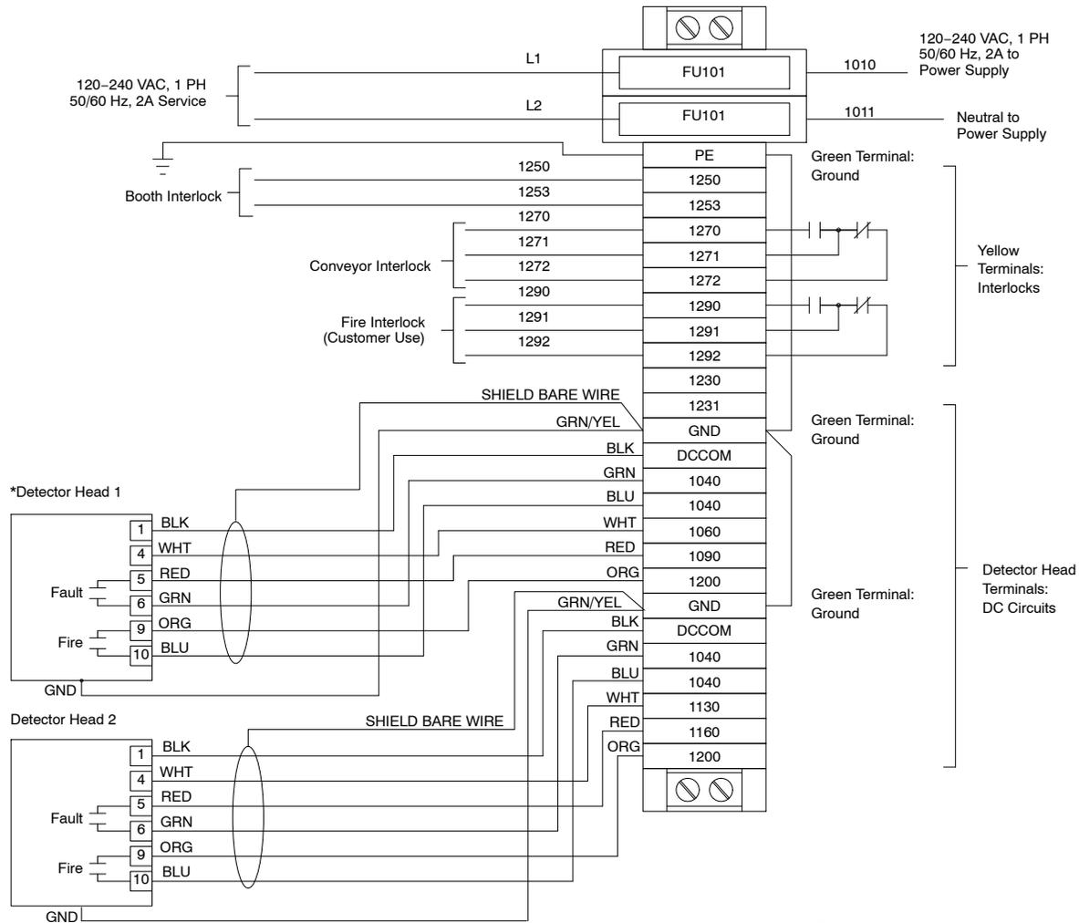
\* For single detector head systems jumper from terminals 1040 to 1160 and from 1230 to 1231
