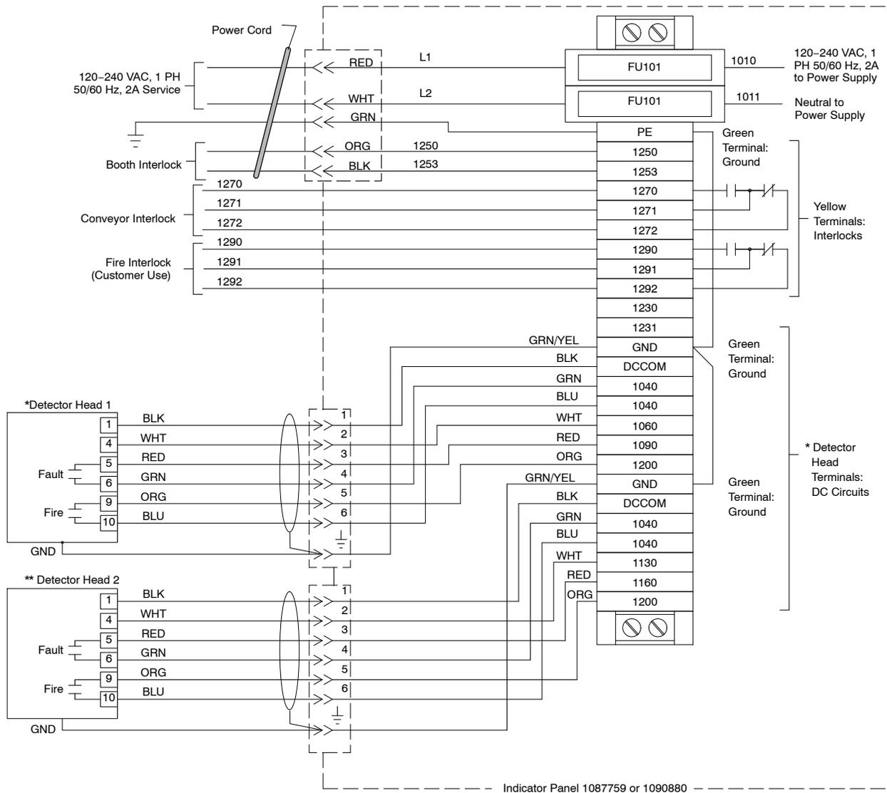
\* For single detector head systems (panel 1090880 jumper from terminals 1040 to 1160 and from 1230 to 1231.
