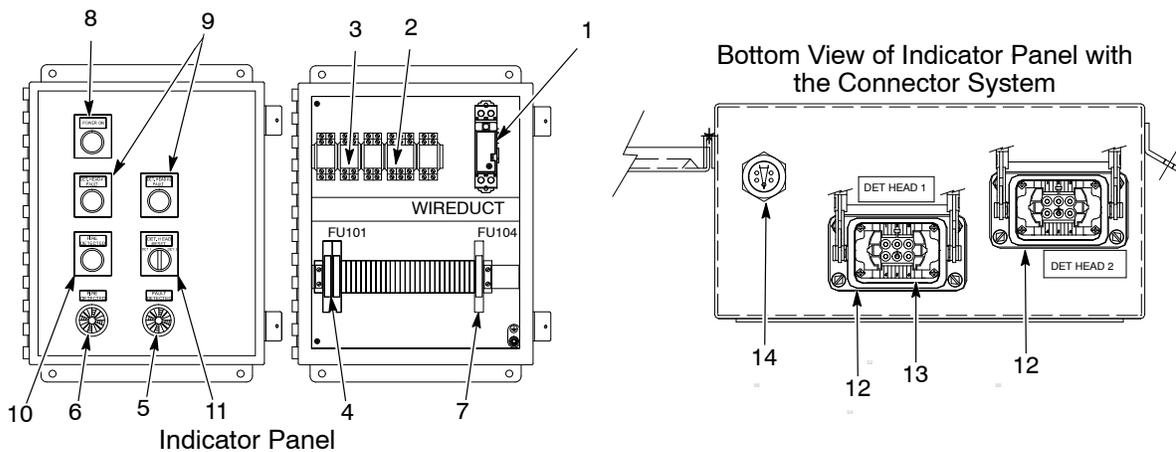
Figure 11 Indicator Panel Parts
