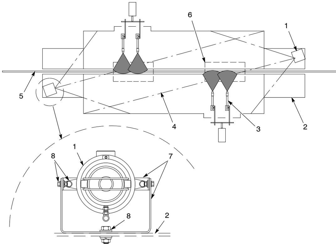
Figure 3 Fire Sensors and Light Test Source Installation Side View
