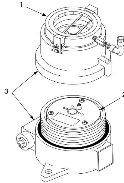
Figure 2 Detector Head Components
