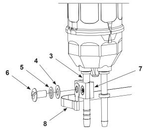
Figure 2 Install Antistatic Tubing Grounding Kit
