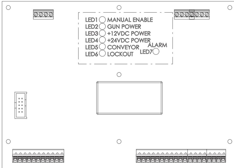
Figure 5-6 Location of LEDs on Relay Board
