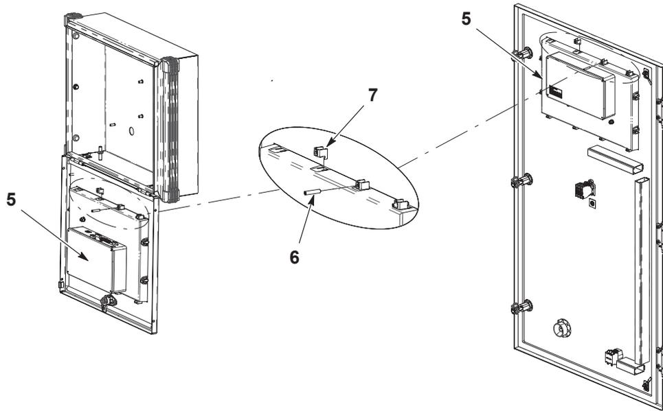
Figure 6-4 Replacing Touchscreen
