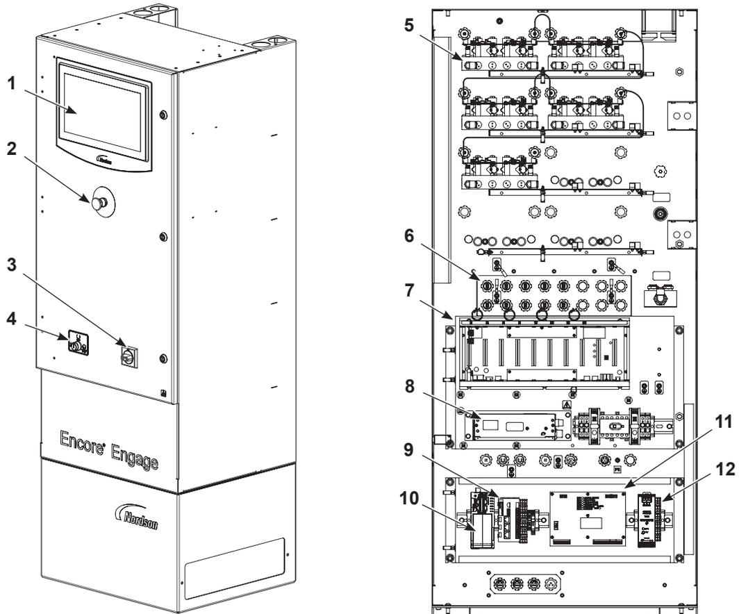
Figure 2-2 Engage Main Console and Pedestal Internal Components
