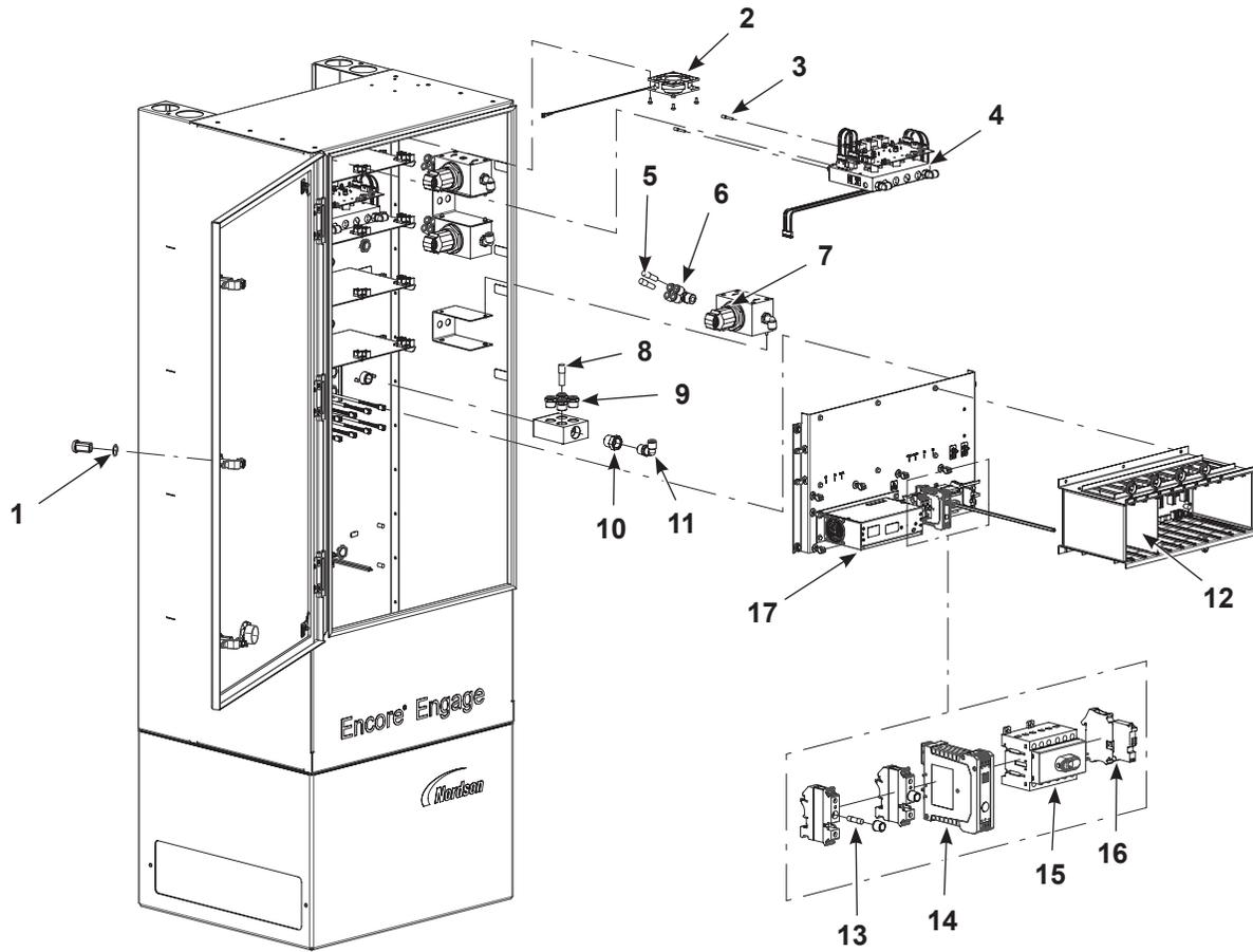
Figure 7-10 Auxiliary Controller Components 1 of 2
