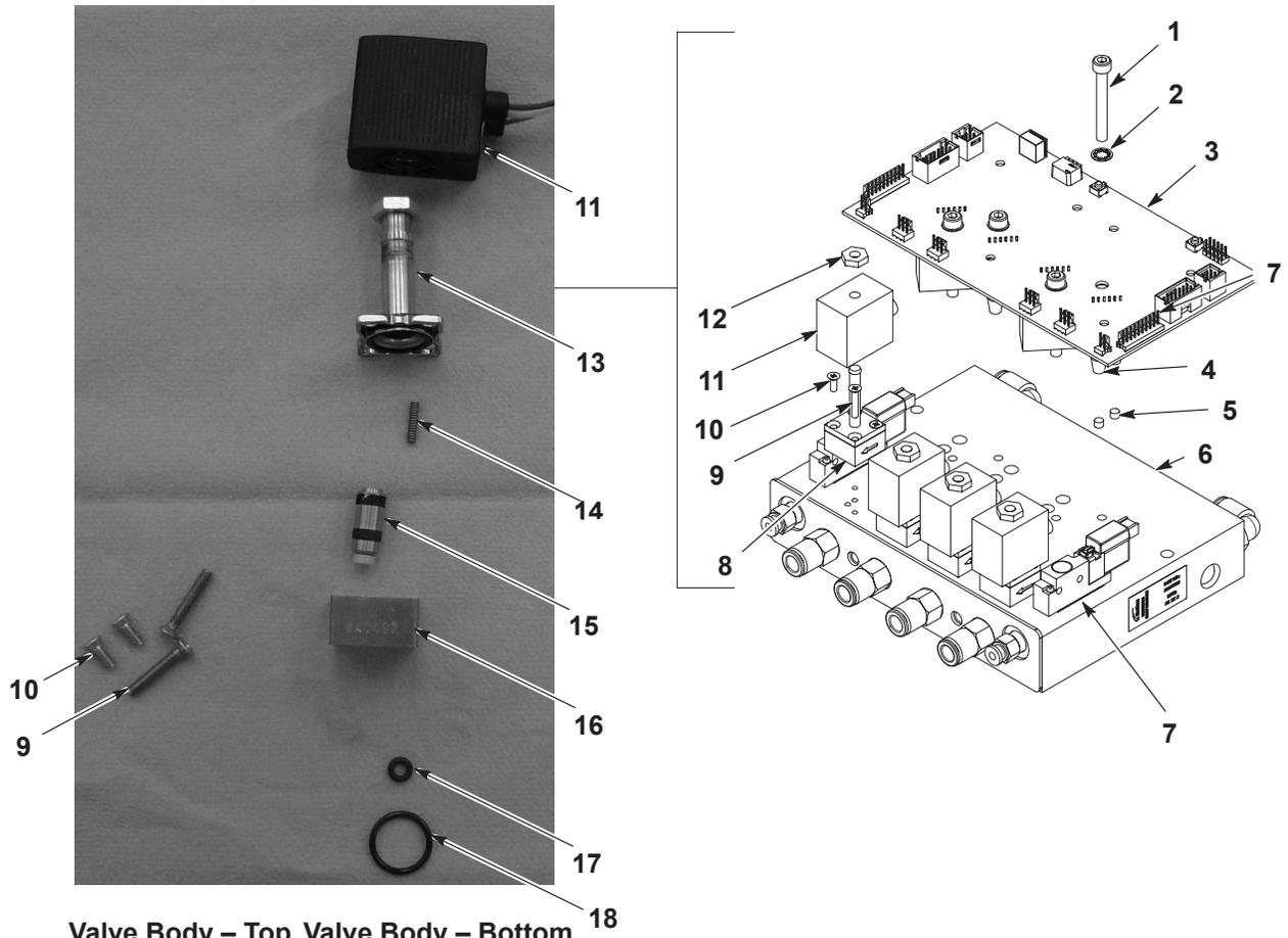
**Valve Body – Top Valve Body – Bottom**
