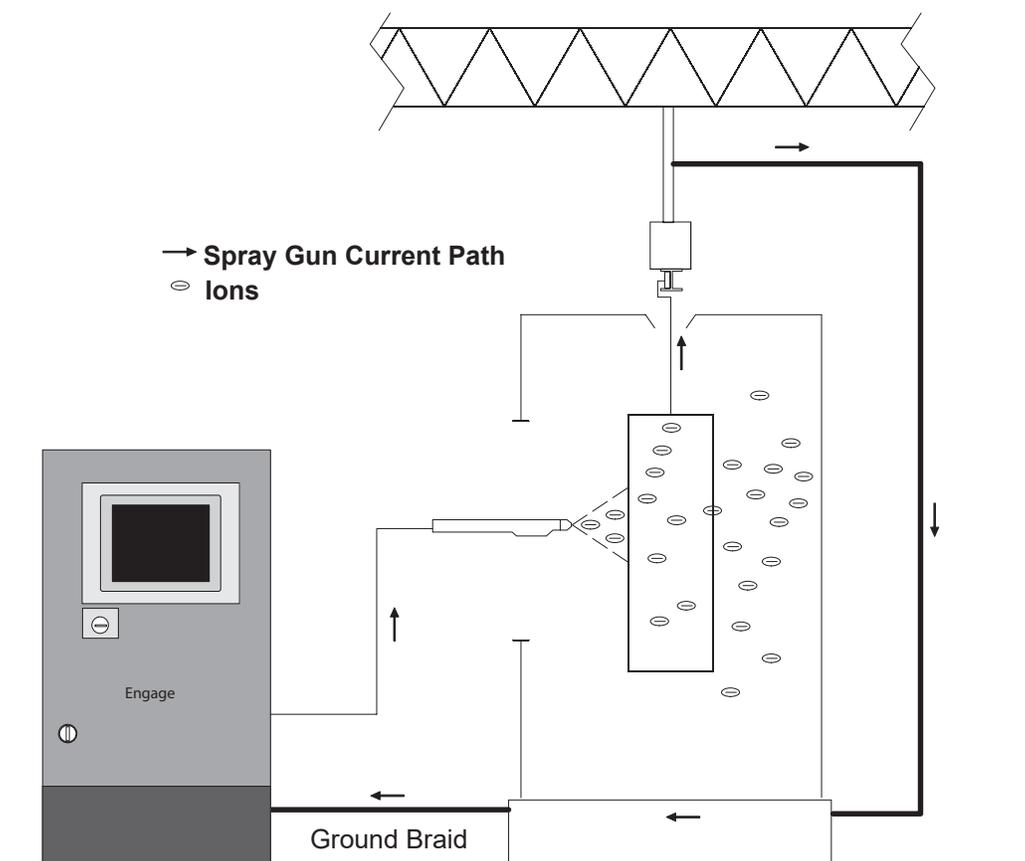
Figure 3-9 Electrostatic Current Path
