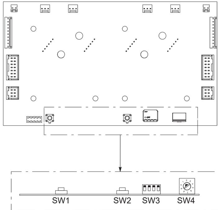
Figure 5-2 Dual Pump Control Board
