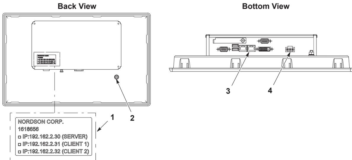
Figure 6-3 Touchscreen IP Label and Connections
