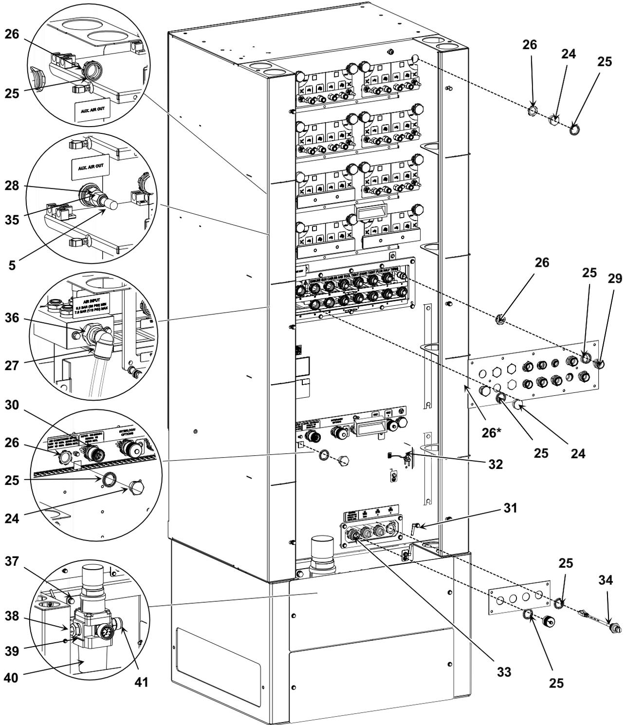
Figure 7-6 Main Controller for Remote Display Components 2 of 2
