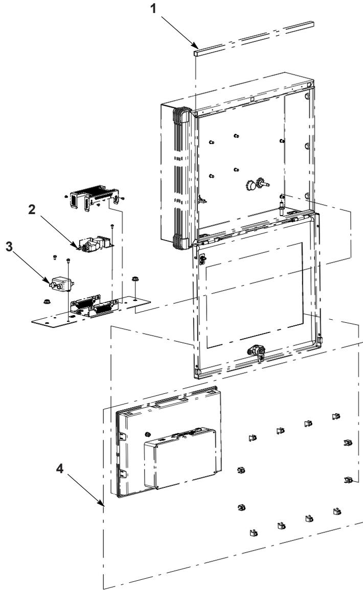
Figure 7-9 Remote Display Components
