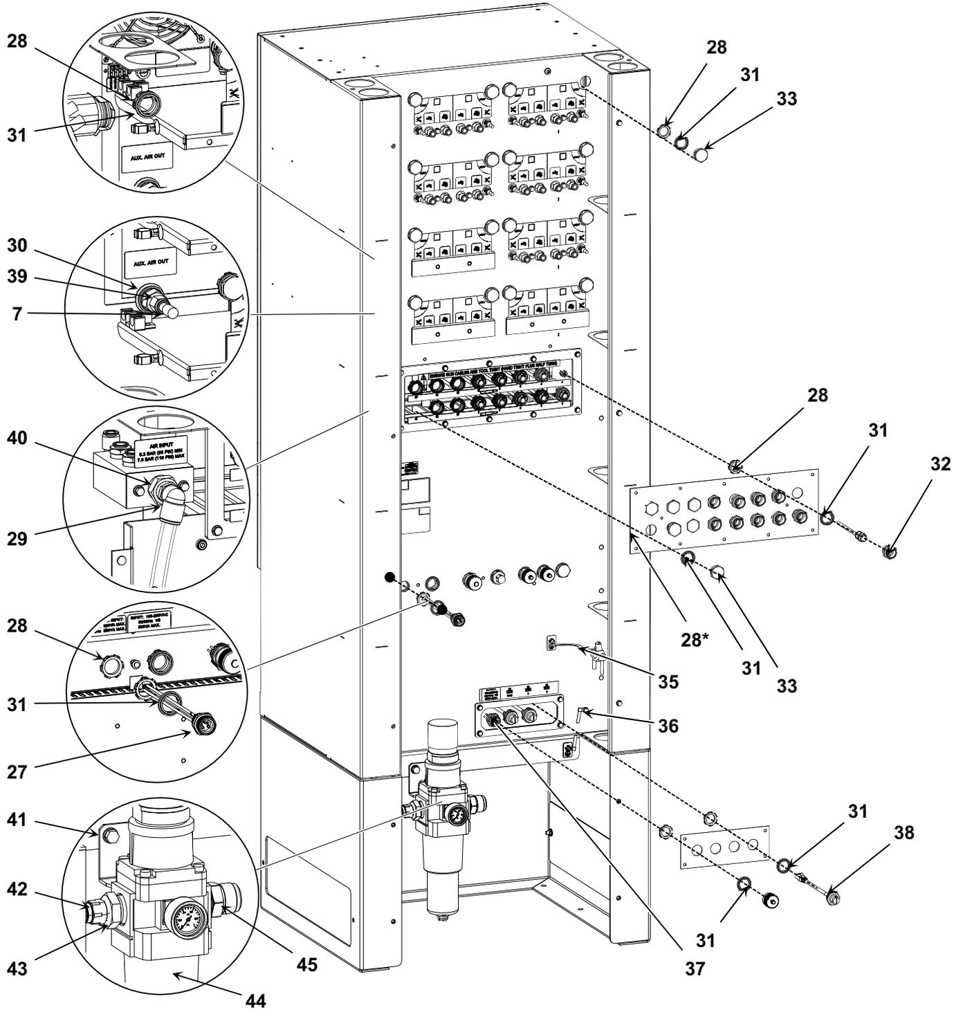
Figure 7-8 Main Controller for Remote Display Components 2 of 2
