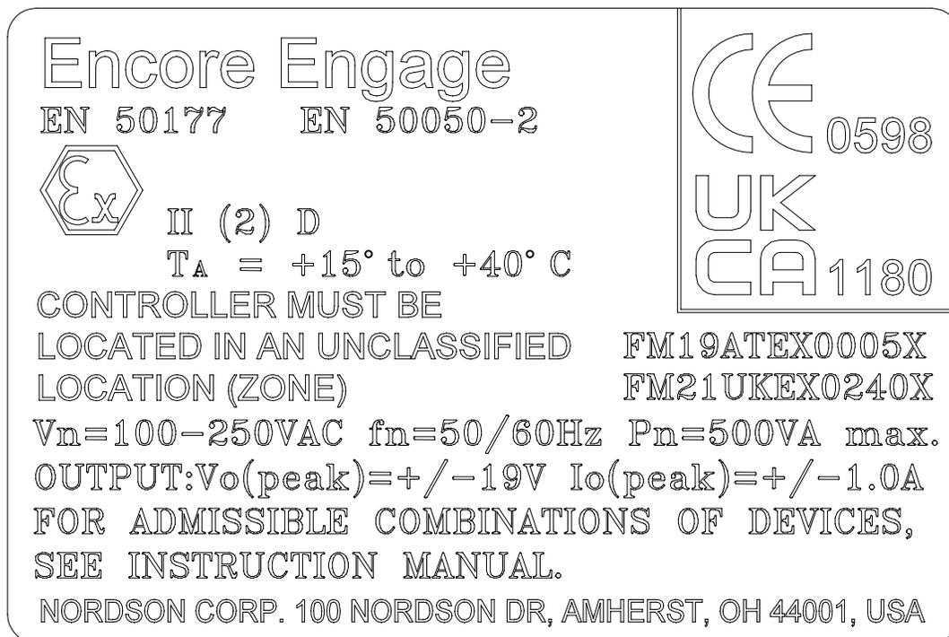
Figure 2-4 Label for CE ATEX and UKCA Approval (On Main and Auxiliary Cabinets)
