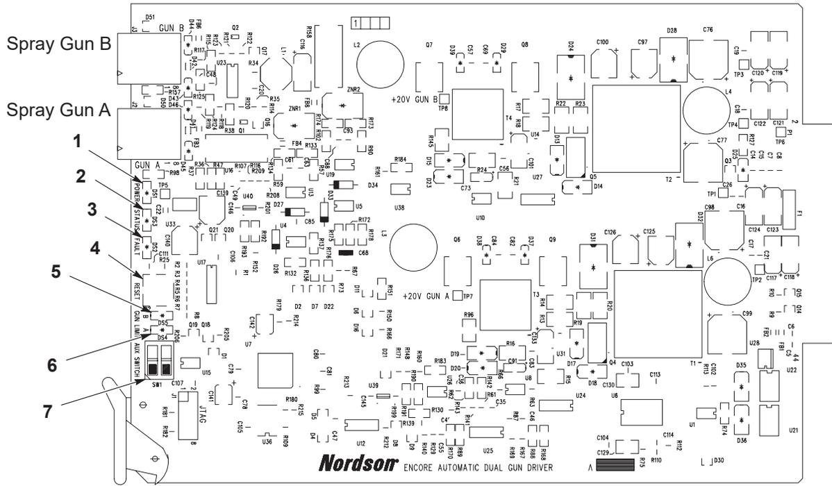
Figure 5-1 Spray Gun Control LEDs and Switches
