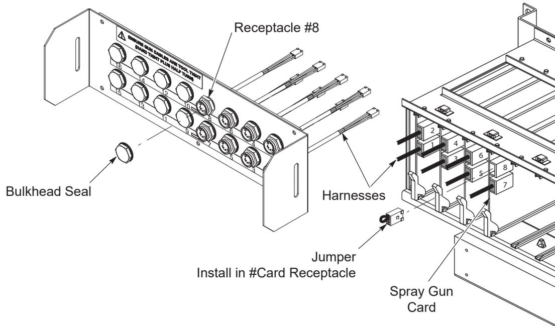
Figure 3-11 Seal and Jumper Installation – Example Showing 8-Spray Gun System Using Seven Spray Guns
