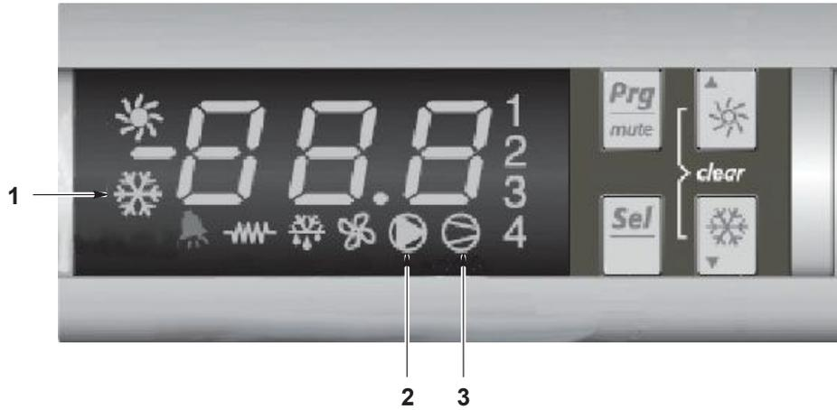
Figure 4-1 Air Conditioner Display LEDs
