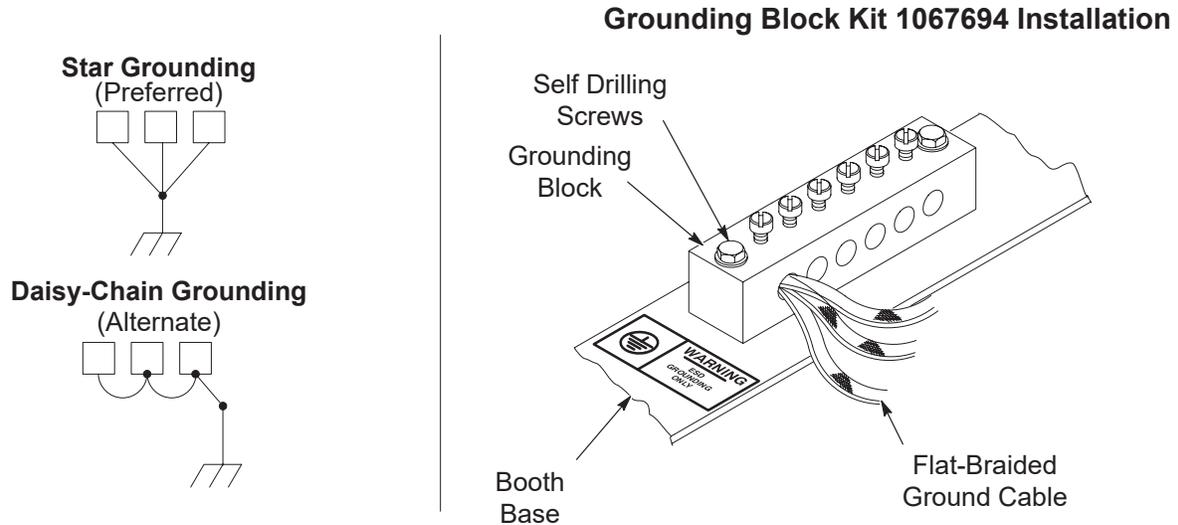
Figure 3-10 ESD Grounding Procedures and Equipment
