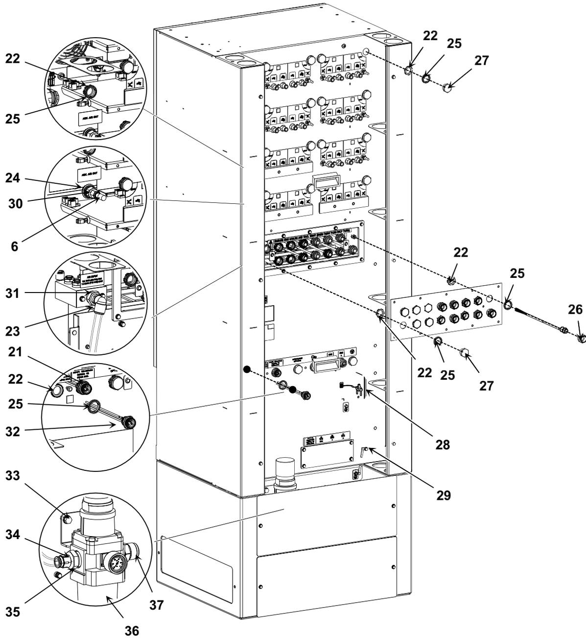
Figure 7-13 Auxiliary Controller Components with Air Conditioner 2 of 2
