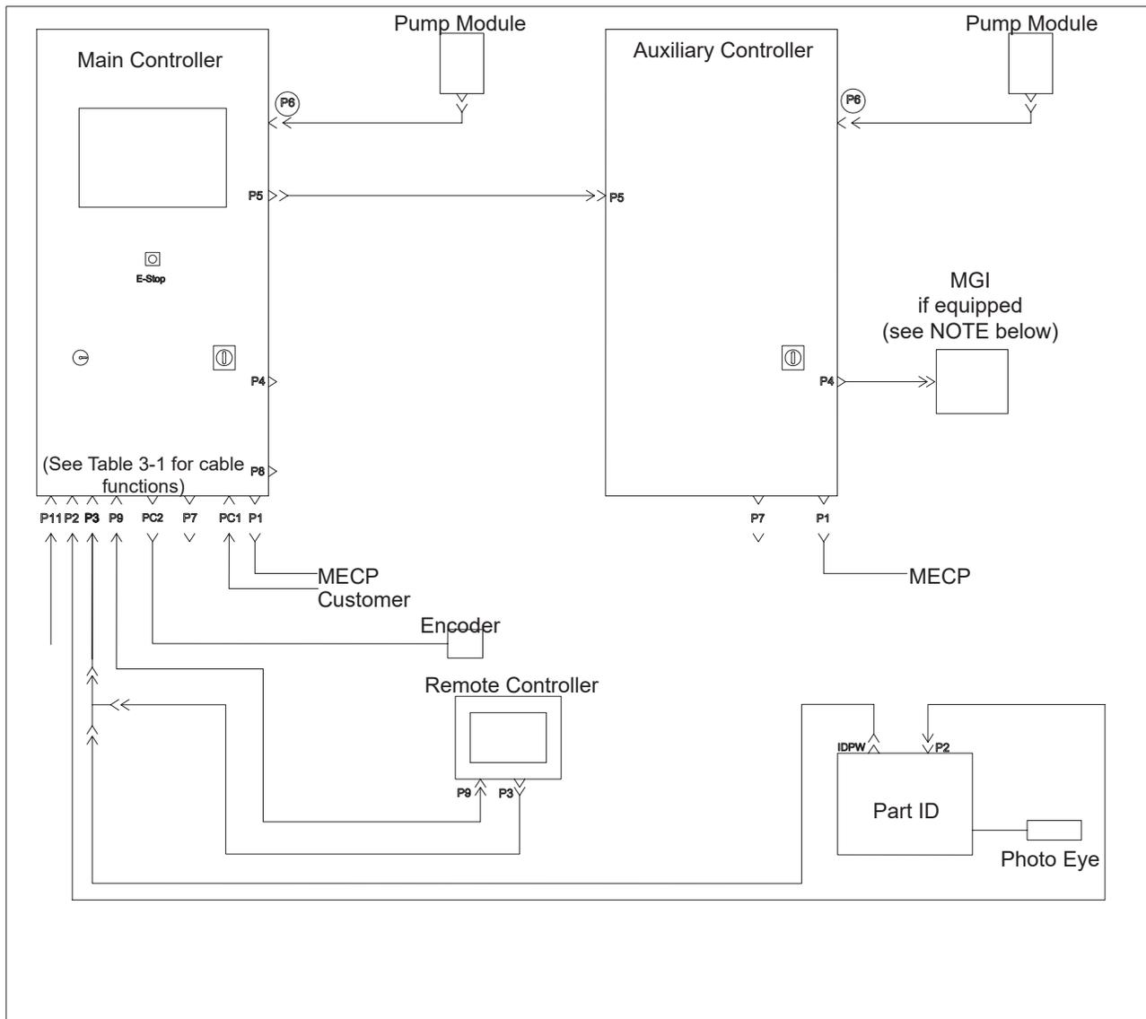
Figure 3-1 Typical System Interconnect Cable Connections
