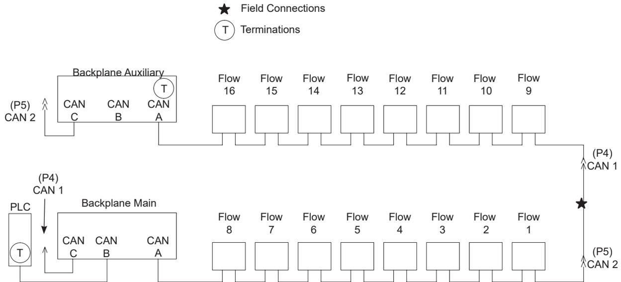
Figure 3-5 CAN Network Cable Connections
