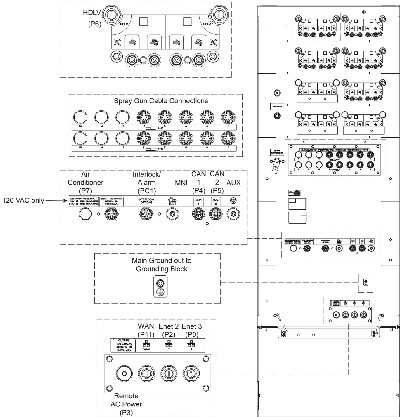
Figure 3-2 Rear Panel of Cabinet (Cover Removed)
