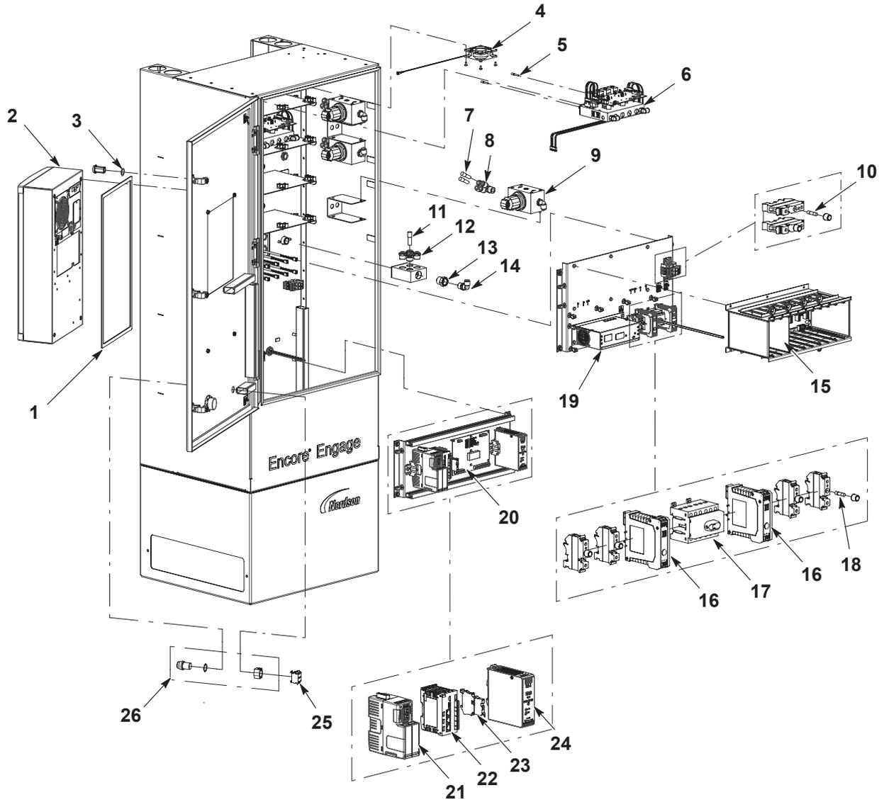
Figure 7-7 Main Controller for Remote Display Components with Air Conditioner 1 of 2
