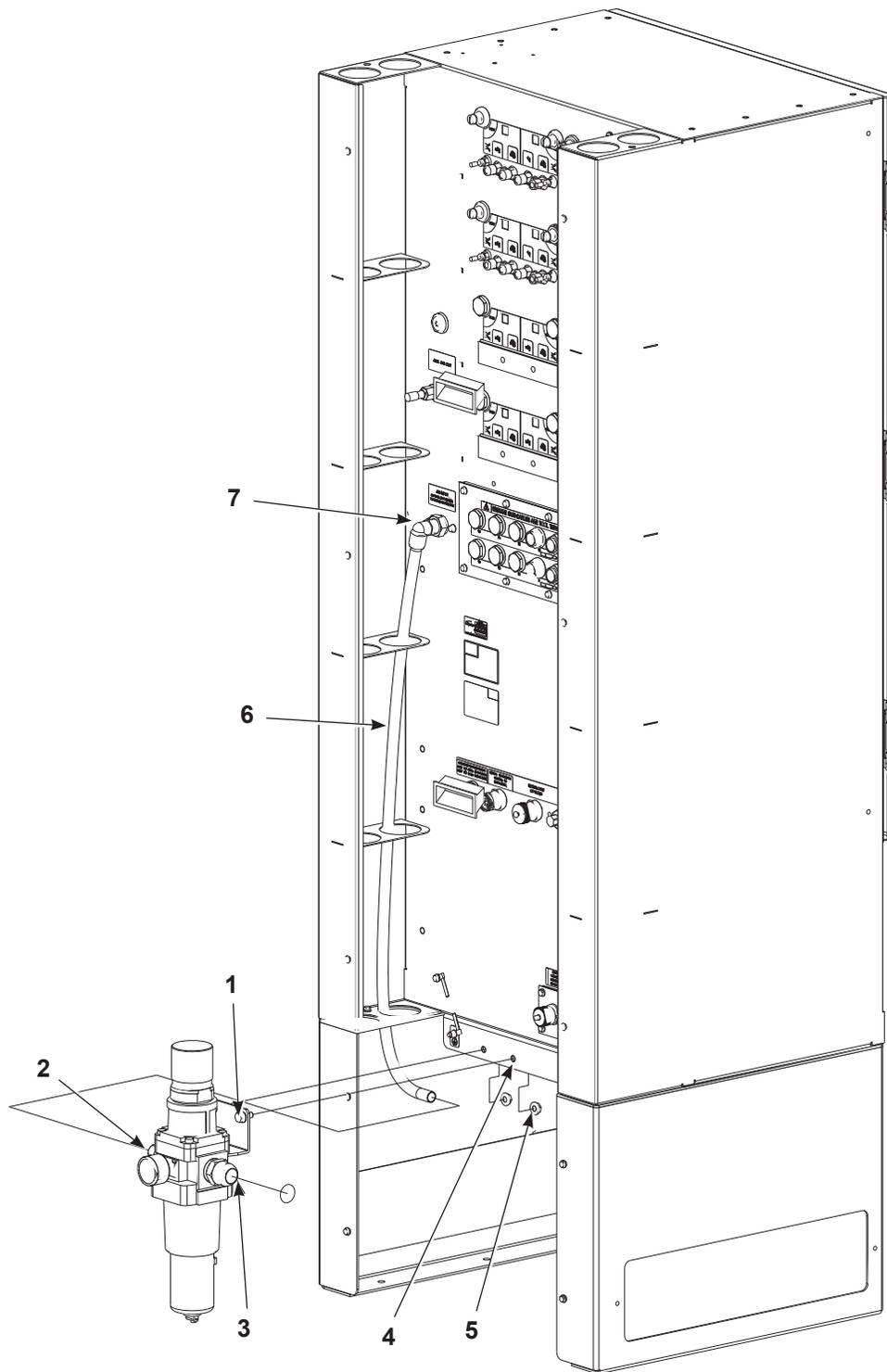
Figure 3-4 Encore Engage External Controller with Optional Air Prep Kit
