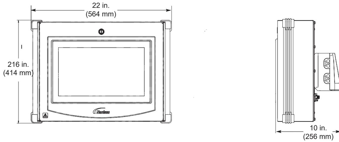
Figure 2-8 Remote Controller Touchscreen Interface Dimensions
