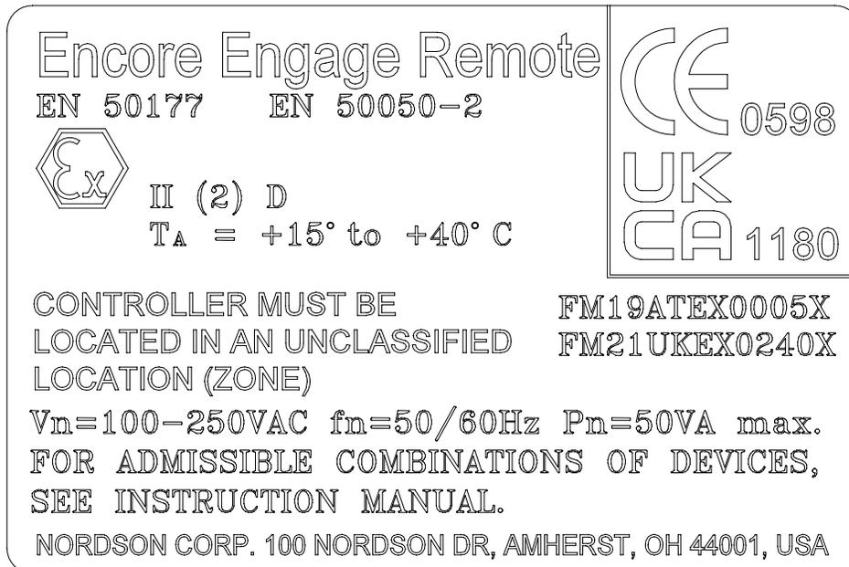
Figure 2-5 Label for CE ATEX and UKCA Approval (On Remote Display)
