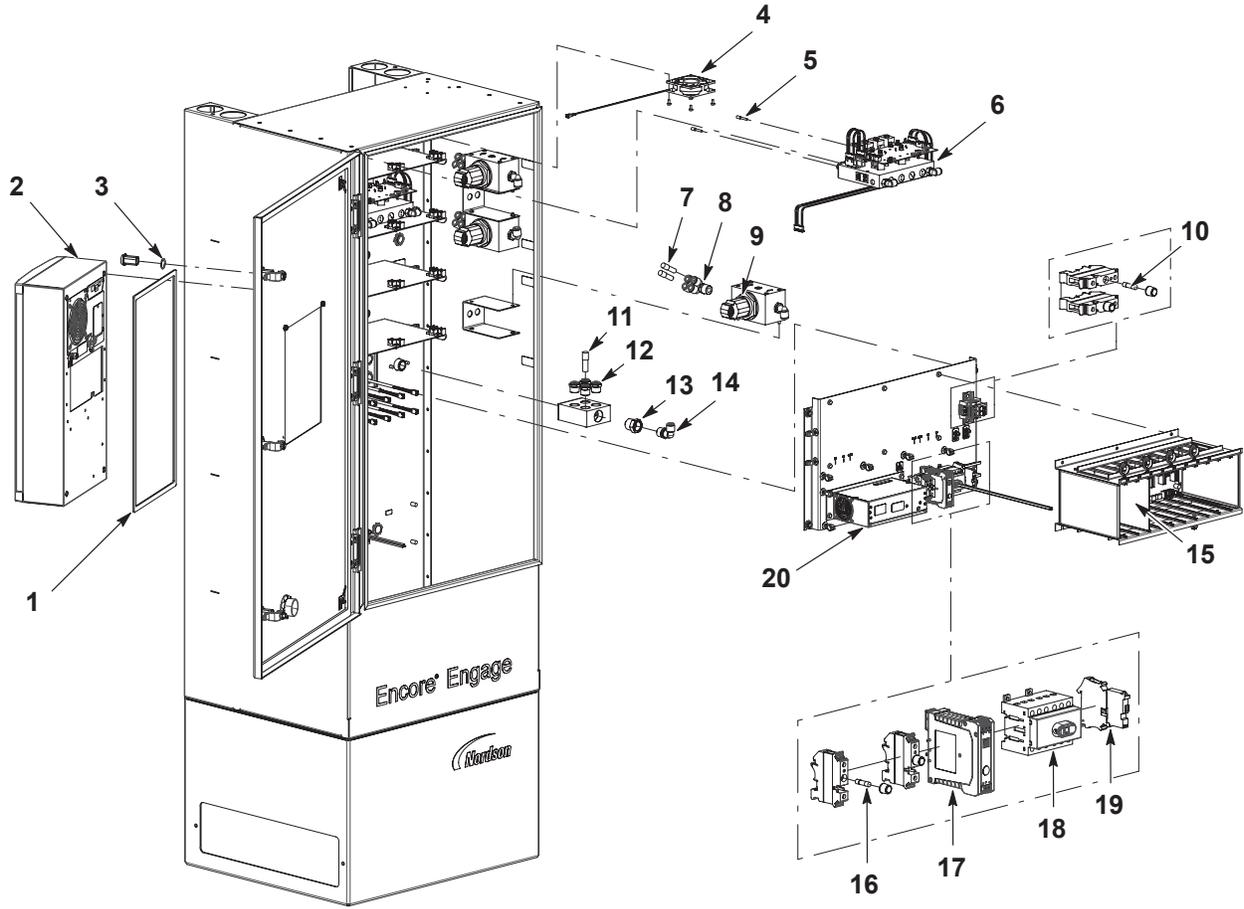
Figure 7-12 Auxiliary Controller Components with Air Conditioner 1 of 2
