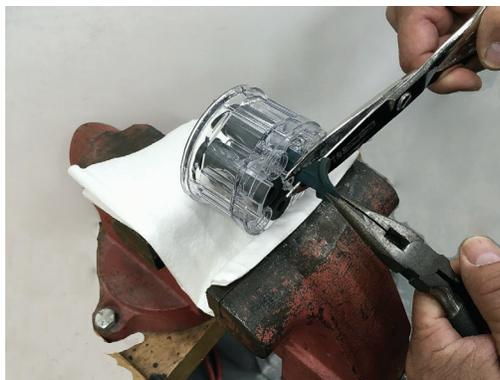
Figure 6-17 Pinch Valve Removal
