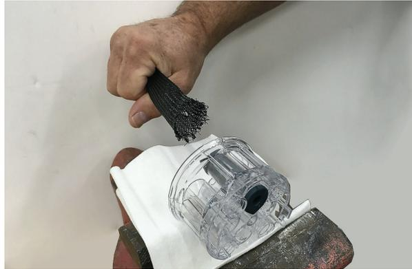
Figure 6-20 Pulling Pinch Valve into Valve Body
