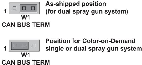
Figure 10 CAN BUS TERM Jumper Settings
