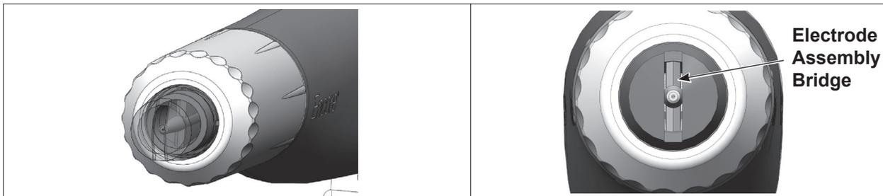
Figure 6 Correct Nozzle Orientation
