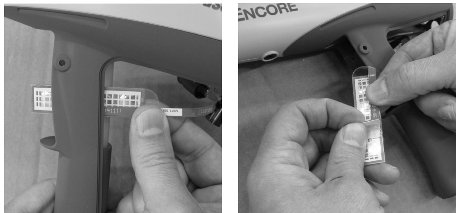
Figure 6-10 Installing the Trigger Switch – Steps 1 and 2
