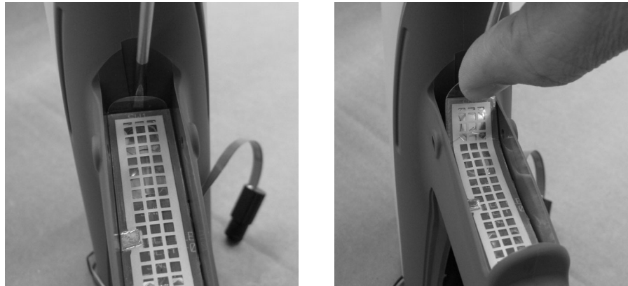
Figure 6-9 Removing the Trigger Switch from the Handle
