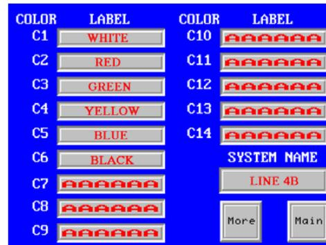
Figure 6 Color Controller Button Label Screen
