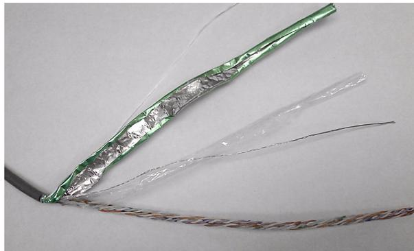
Figure 3-8 Ethernet Cable Termination, Steps 3-4
