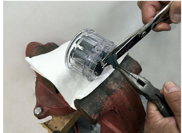
Figure 29 Pinch Valve Removal
