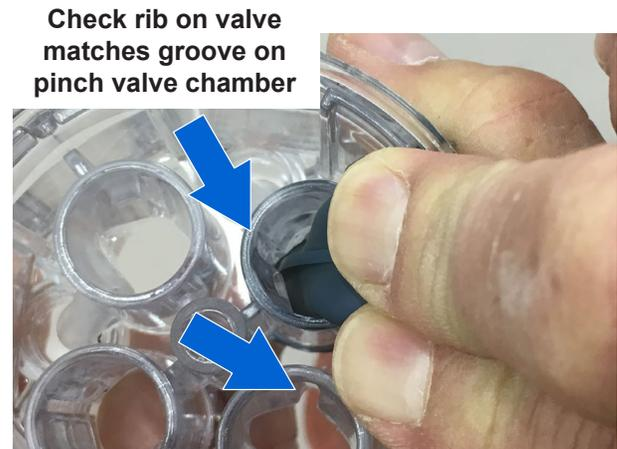
Figure 33 Checking Rib and Groove Alignment
