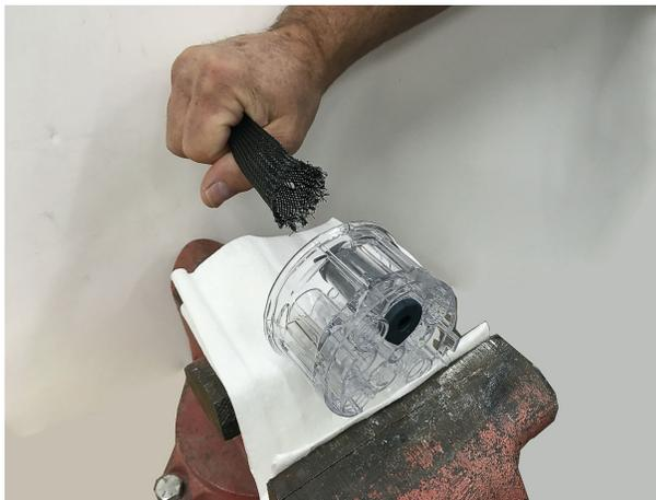
Figure 32 Pulling Pinch Valve into Valve Body
