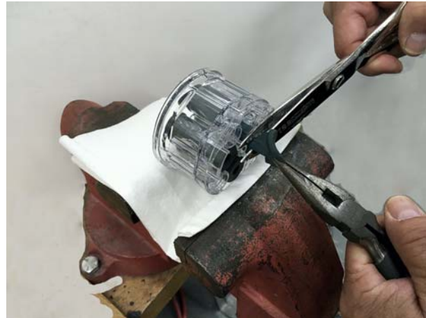
Figure 3 Pinch Valve Removal
