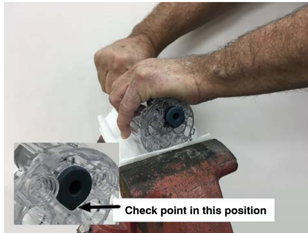
Figure 6 Pulling Pinch Valve into Valve Body
