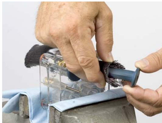
Figure 11 Inserting Pinch Valve into Pump Pinch Valve Tool
