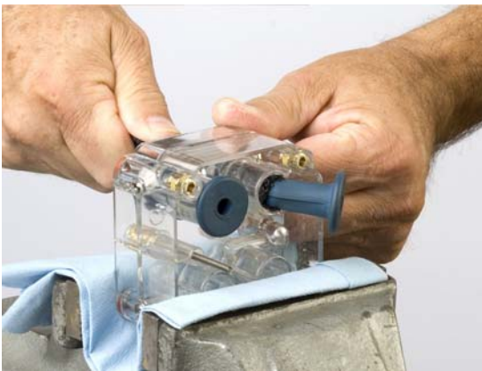
Figure 13 Pulling Pinch Valve into Valve Body
