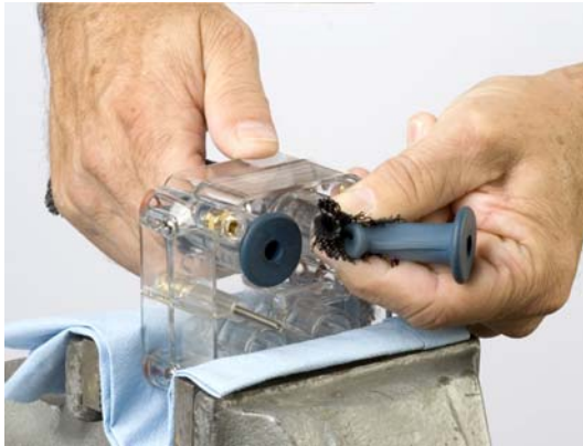
Figure 12 Pinching Flat Pinch Valve Up Flange
