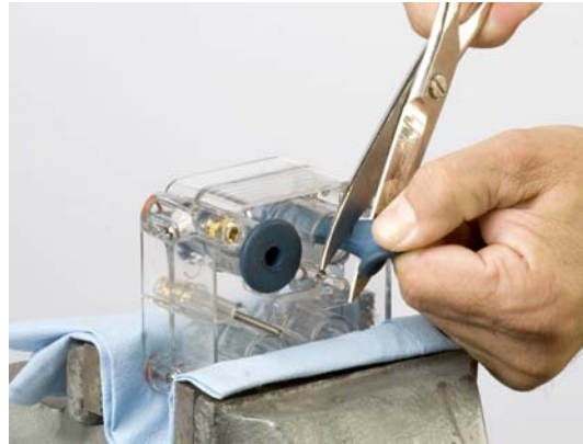
Figure 10 Pinch Valve Removal
