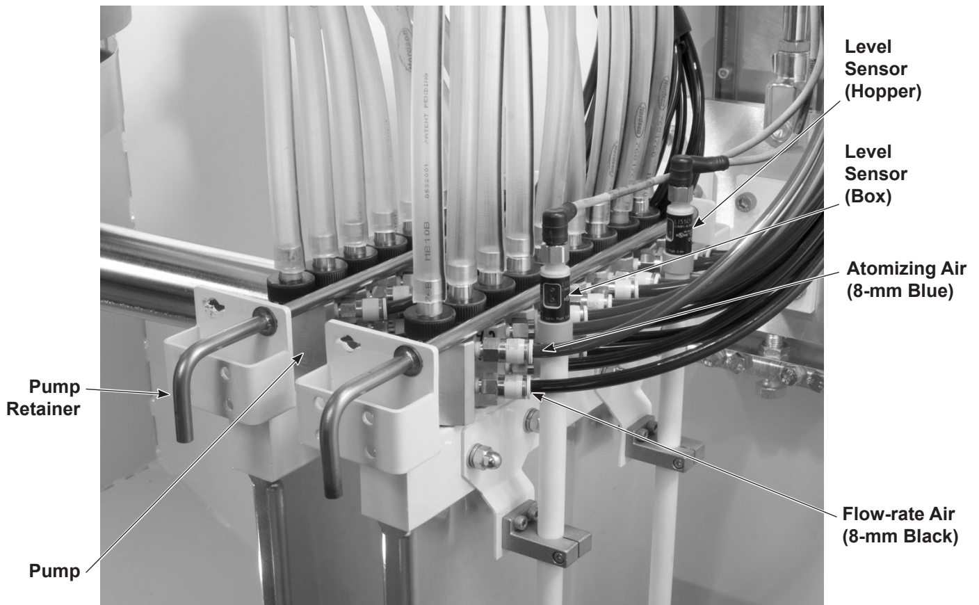
Figure 3-2 Pump, Air Tubing, and Powder Feed Hose Installation
