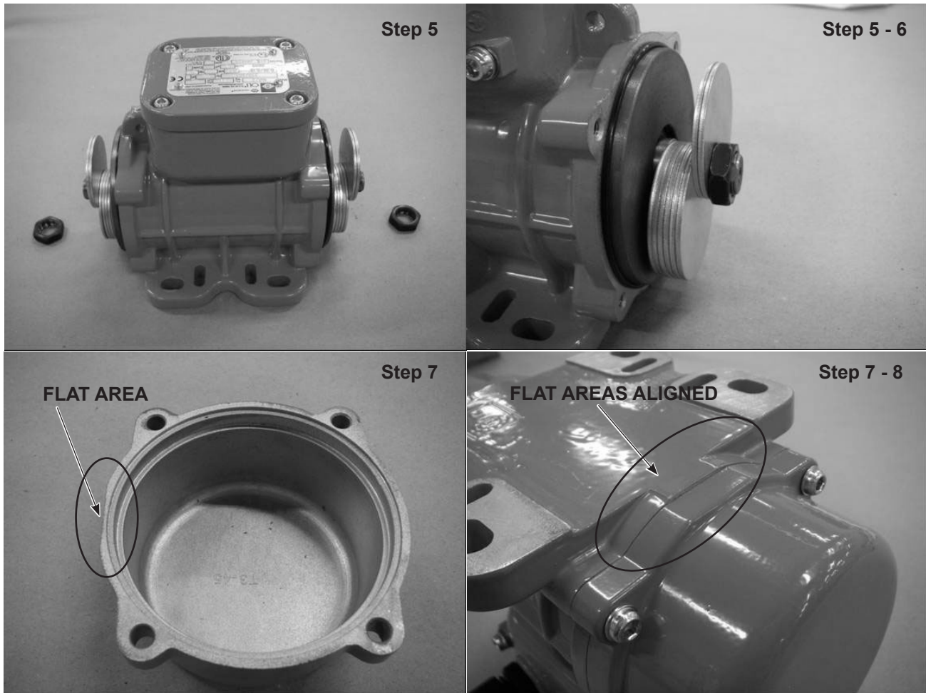
Figure 8-15 Vibrator Weight Adjustment, 60Hz, Steps 5-8
