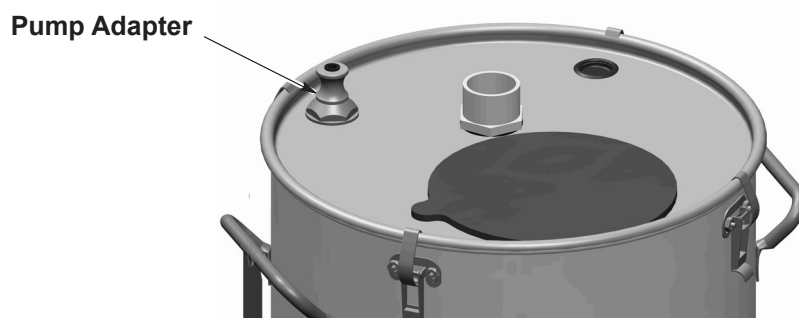
Figure 3-13 Pump Mounting with Adapter on HR or NHR Hoppers
