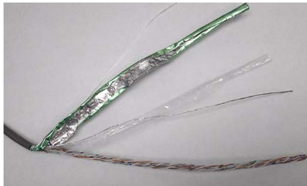
Figure 3-9 Ethernet Cable Termination, Steps 3-4
