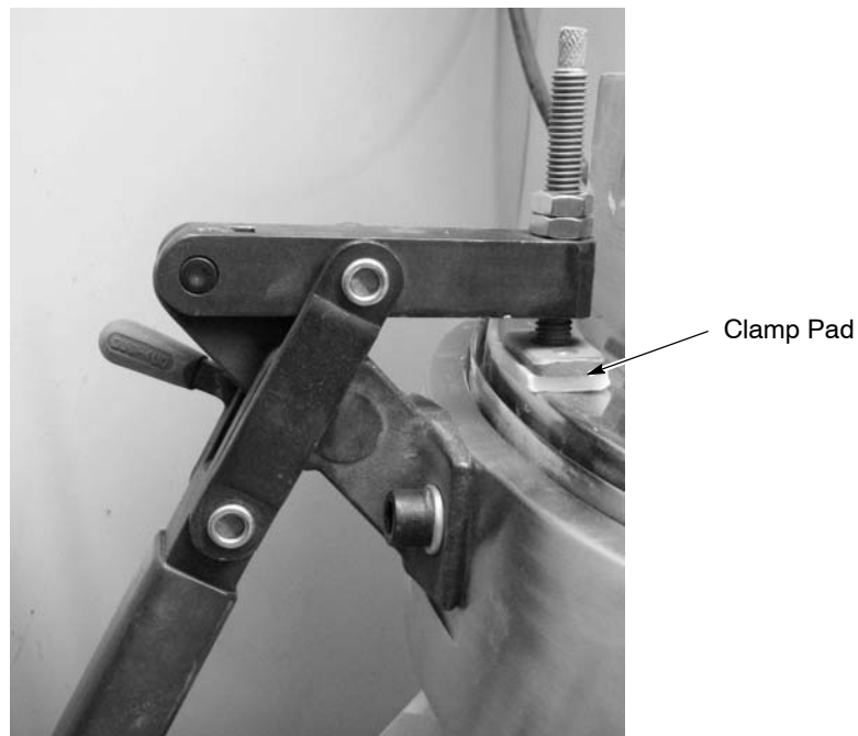
Figure 3 Correct Clamp Pad Position – Clamp Shown Toggled Over-Center
