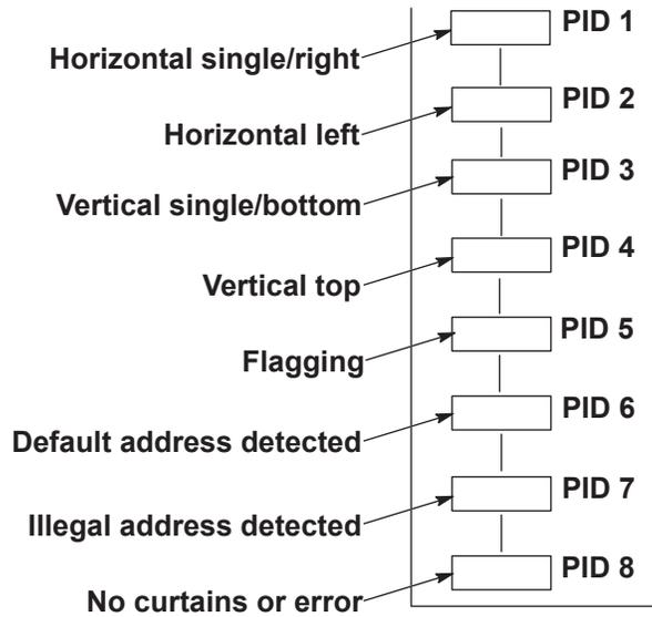
Figure 4 Part ID LEDs
