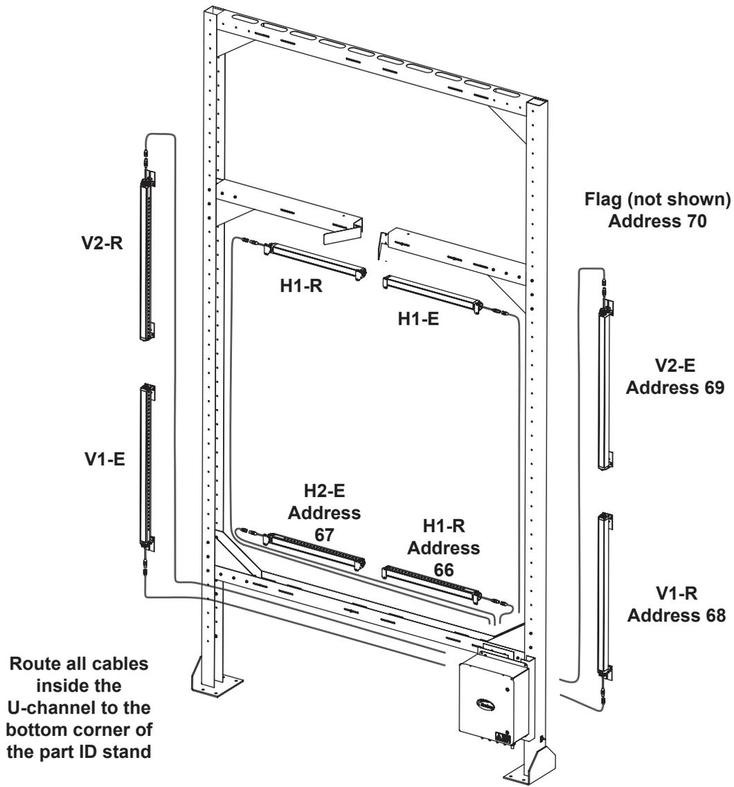
Figure 14 Sensor Location and Cable Routing
