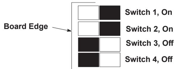
Figure 11 DIP Switch Setting
