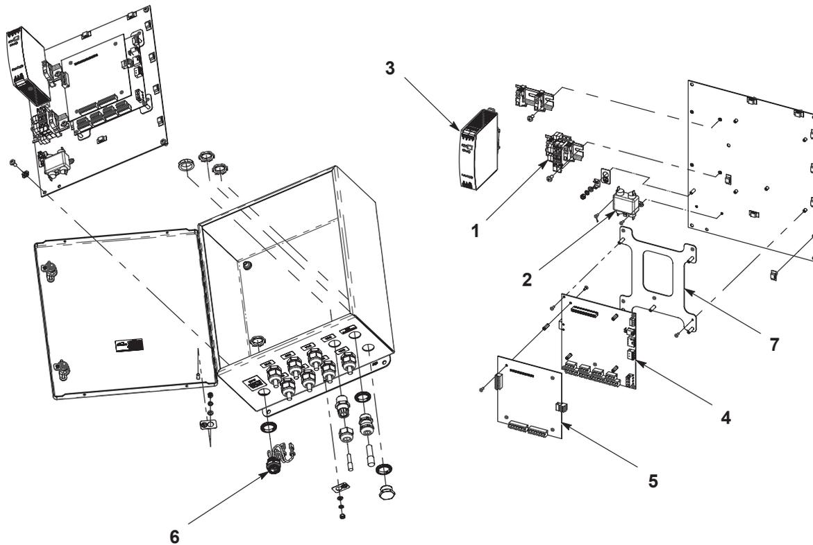
Figure 19 Beam Array Junction Box
