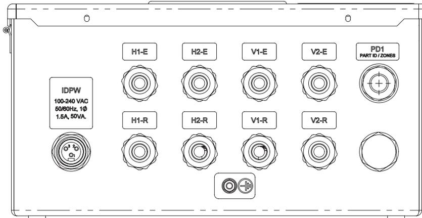
Figure 7 Beam Array Sensor Cable Entrance to Junction Box (outside bottom view)
