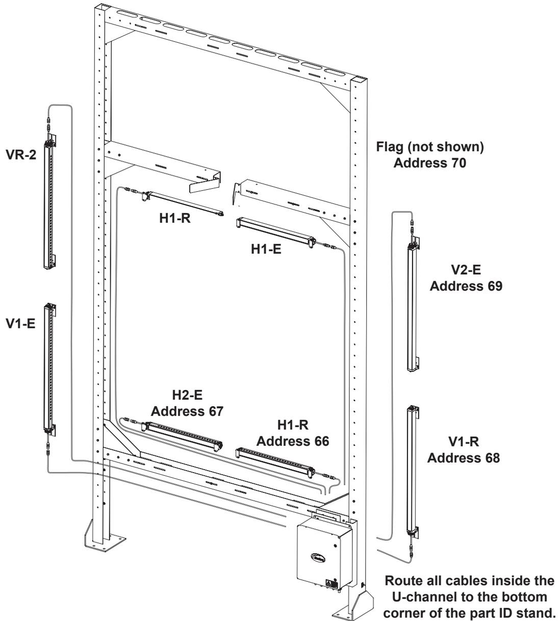
Figure 6 Sensor Location and Cable Routing
