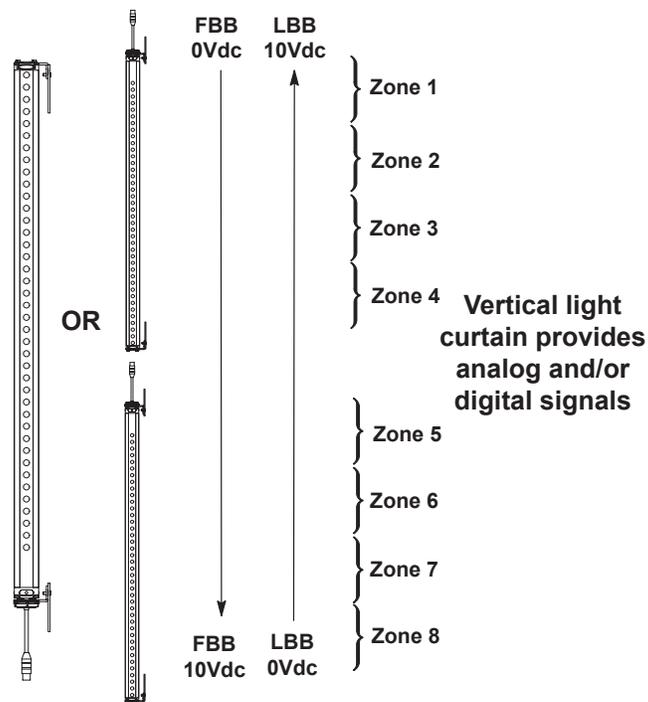
Figure 12 Vertical Beam Array Configuration
