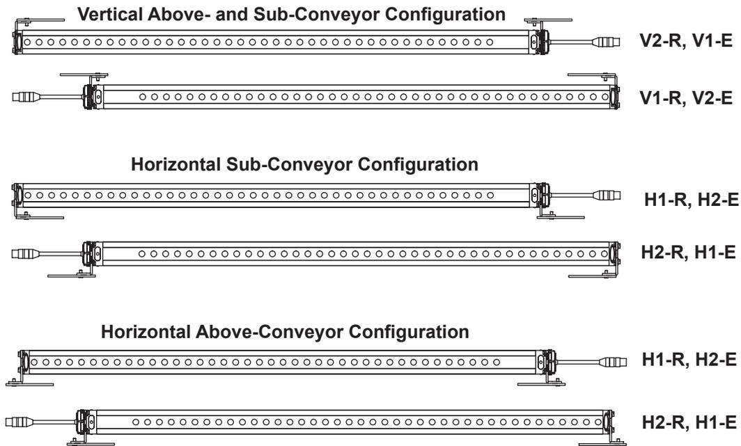
Figure 15 Beam Array Bracket Orientation
