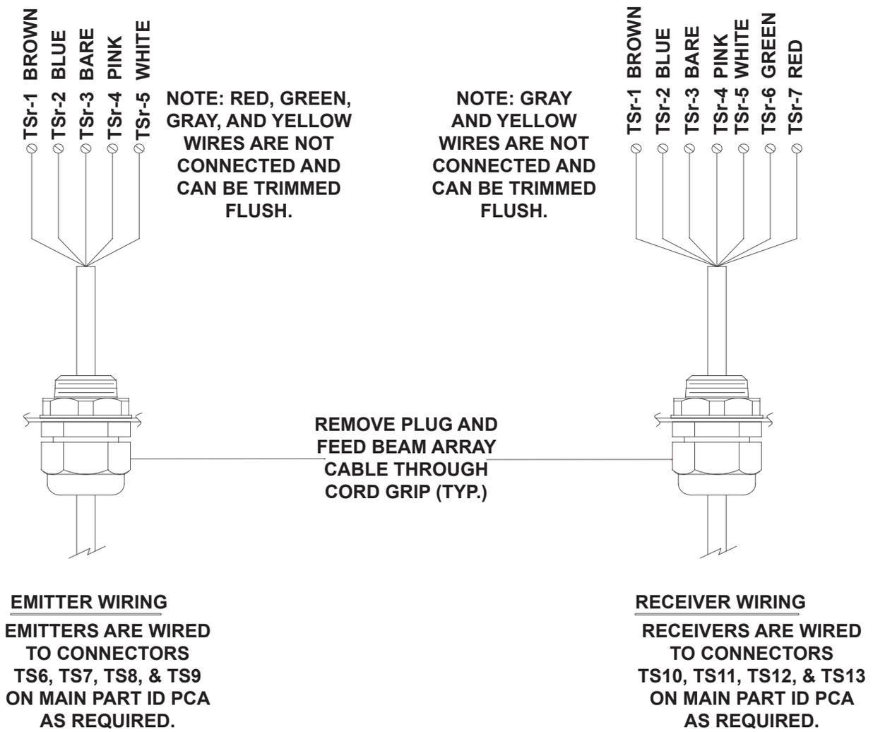
Figure 8 Beam Array Junction Box Wiring
