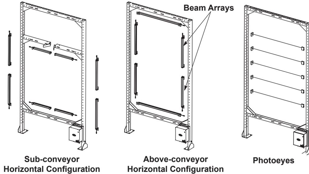
Figure 2 Junction Box with Part ID Stand and Arrays
