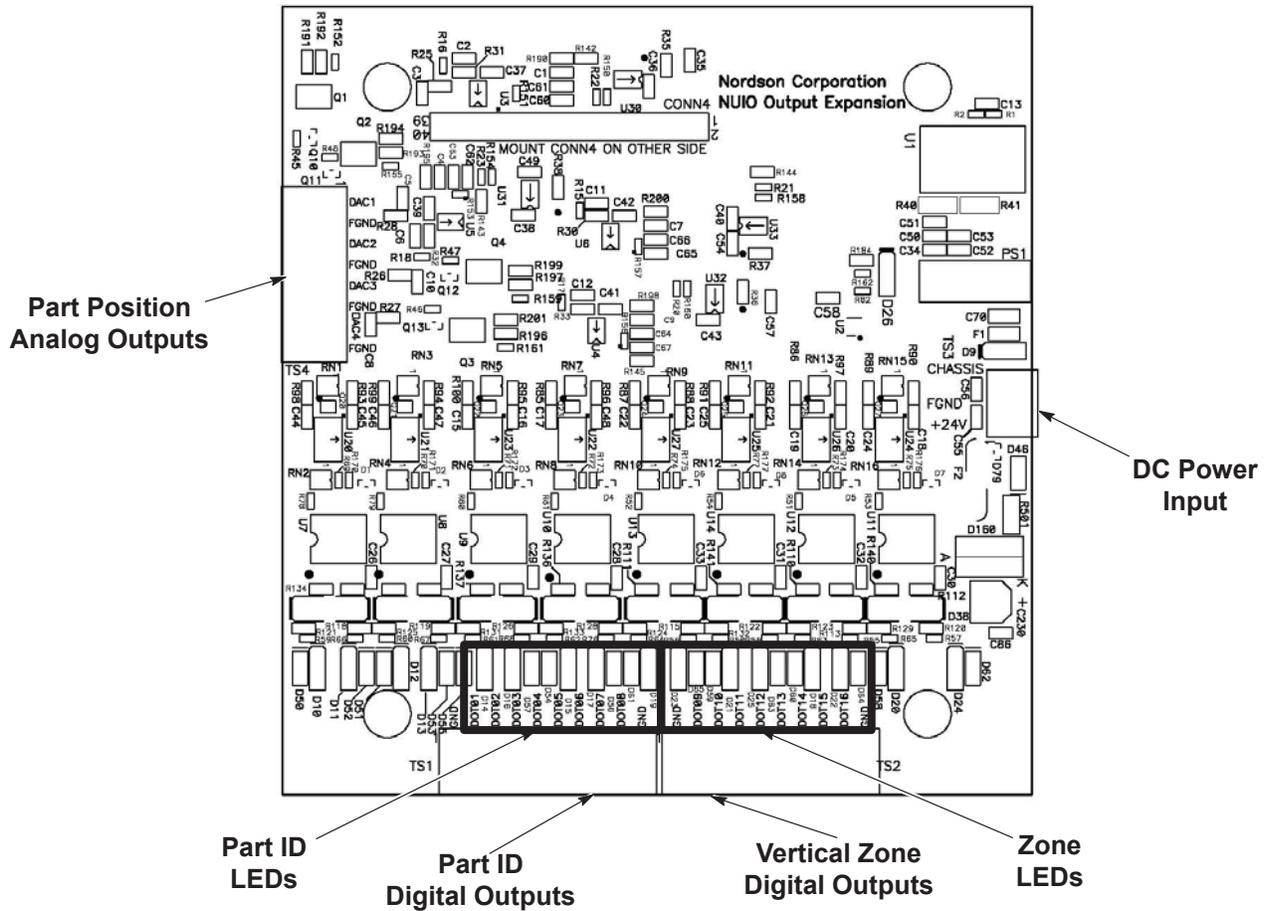
Figure 5 Output Expansion Board
