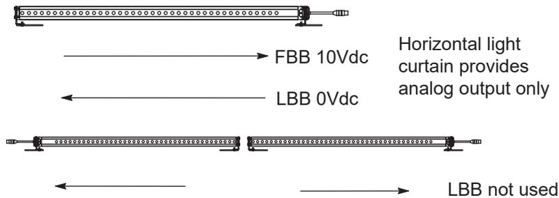
Figure 13 Horizontal Beam Array Configuration
