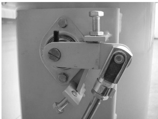
Figure 3-12 Damper Setting, Adjusted Low Flow Position
