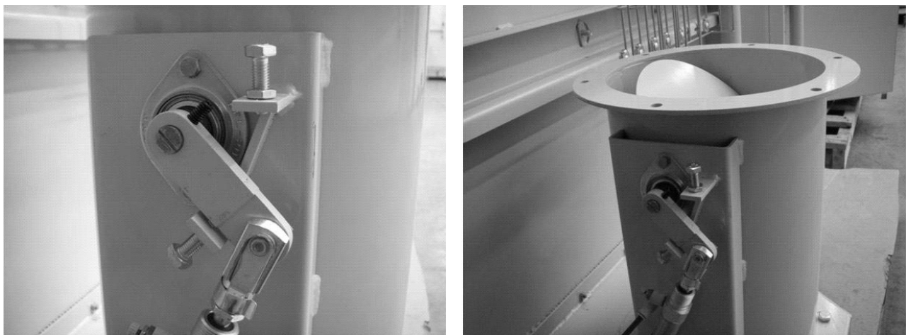
Figure 3-11 Damper Setting, Factory-Set High Flow Position
