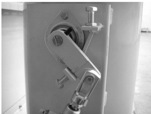
Figure 3-13 Damper Setting, Adjusted High Flow Position
