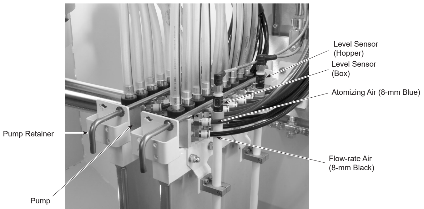
Figure 3-3 Pump, Air Tubing, and Powder Feed Hose Installation
