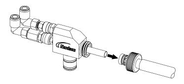
(2) Remove the throat from the pump body. Insert the gage into the throat.
