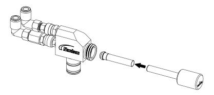
(3) If the gage does not bottom out on the face of the throat, the throat is not worn beyond limits.
