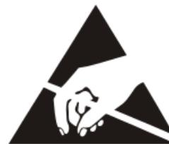
This product has semiconductors that can be damaged by electrostatic discharge (ESD). When handling, take extreme care to prevent damage to the devices.
