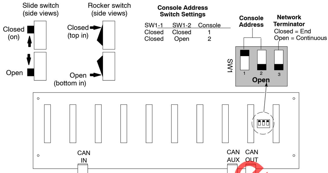
Figure 3-2 CAN Network Connections, Console Addresses, and Termination
