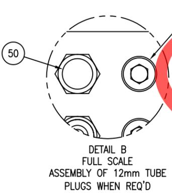
THESE POSITIONS WILL EITHER HAVE A FITTING OR A PIPE PLUG DEPENDING ON NUMBER OF GUNS.
