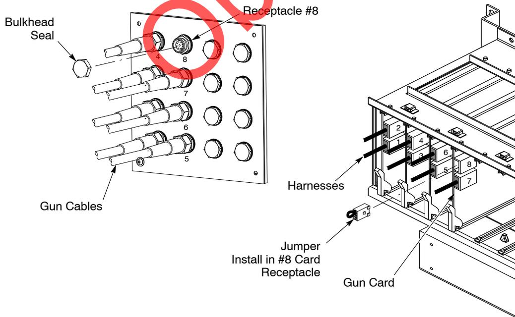
Figure 3-12 Seal and Jumper Installation – Example Showing 8 Gun System Using 7 Guns
