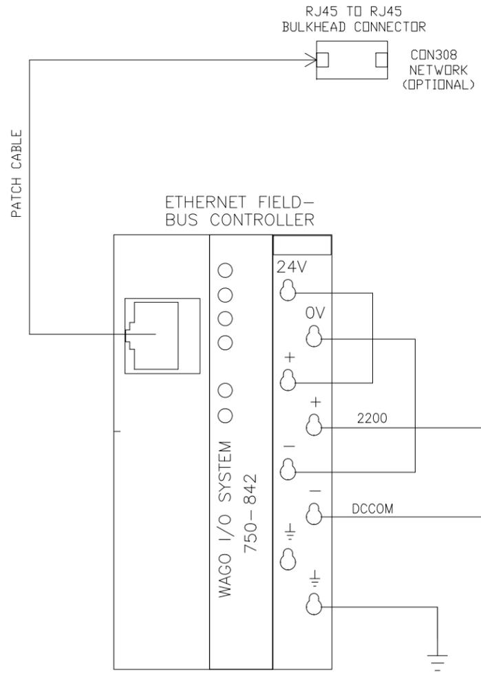
ADD JUMPER, AS INDICATED, TO MATCH MOTION CONFIGURATION TO THE MACHINE CONTROL.
