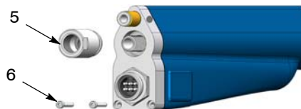
Figure 4 Removing Heat Sink Screws and Lock Nut
