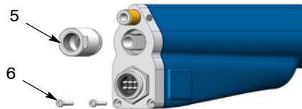
Figure 4 Removing Heat Sink Screws and Lock Nut
