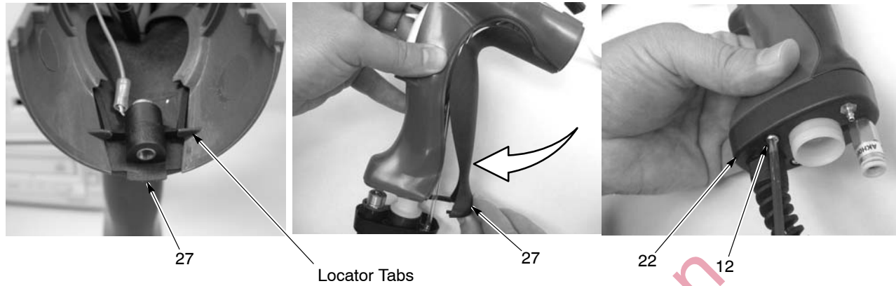
Figure 5-12 Assembling Ground Pad and Base to Handles
