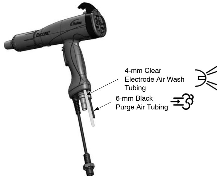
Figure 2-6 Connecting the Purge and Air Wash Tubing to the Spray Gun
