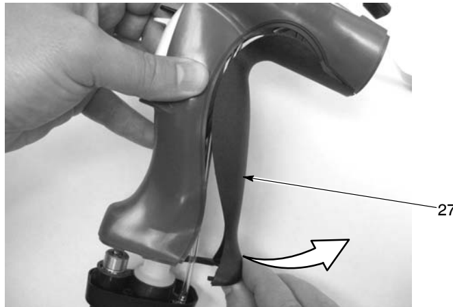
Figure 5-7 Removing the Ground Pad
