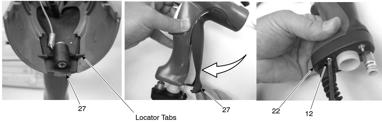
Figure 5-12 Assembling Ground Pad and Base to Handles
