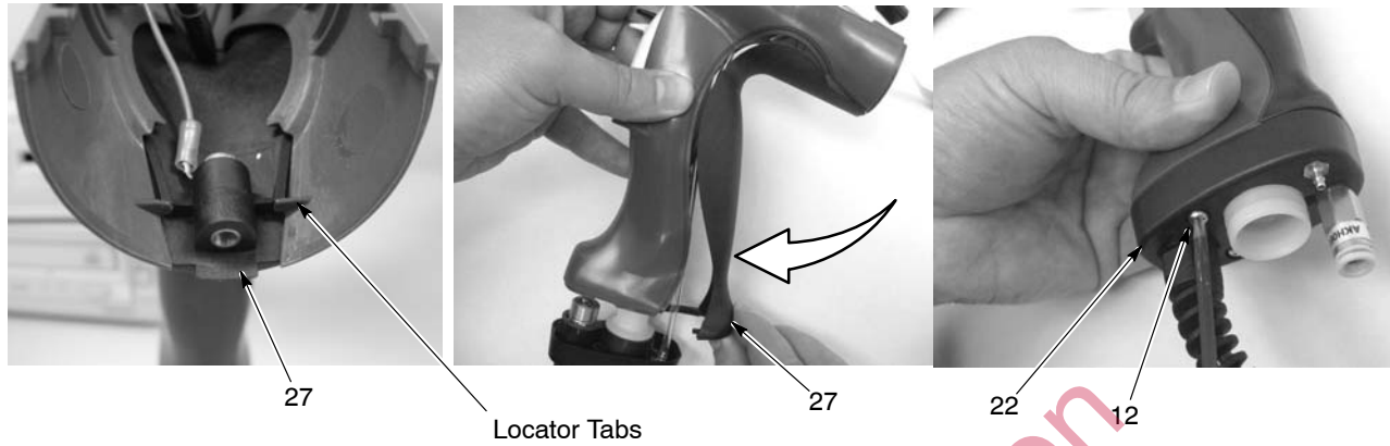
Figure 5-12 Assembling Ground Pad and Base to Handles
