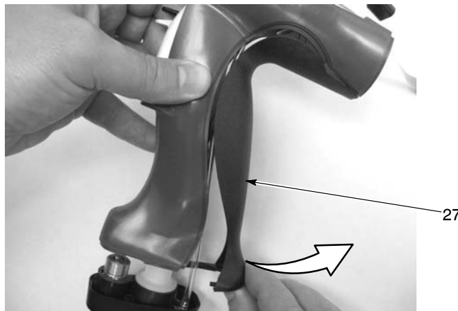
Figure 5-7 Removing the Ground Pad
