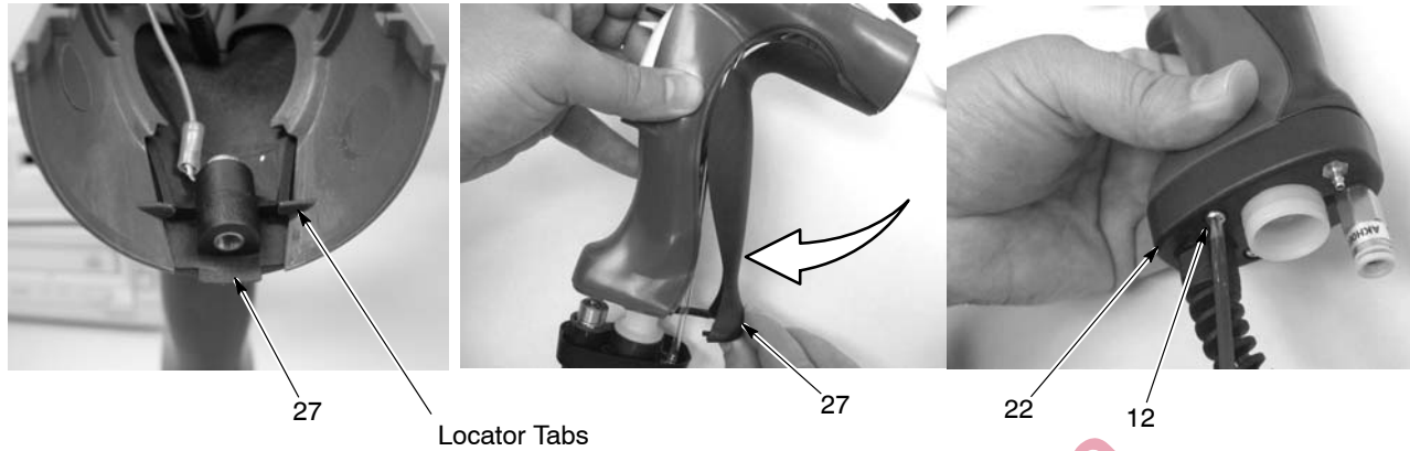
Figure 5-12 Assembling Ground Pad and Base to Handles
