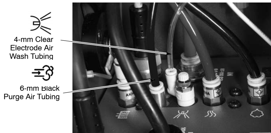
Figure 2-11 Connecting Air Tubing to the Power Unit
