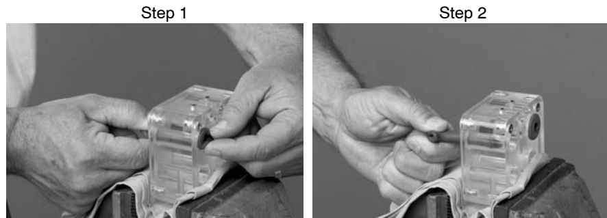
Figure 12 Pinch Valve Removal (Pump Valve Body Shown, Procedure is Same)
