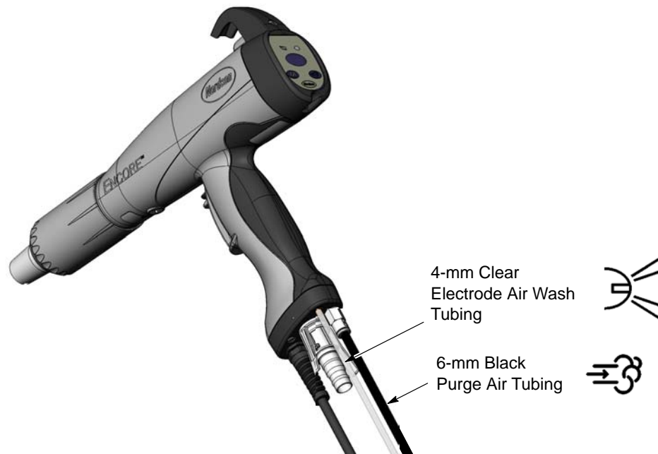
Figure 2-6 Connecting the Purge and Air Wash Tubing to the Spray Gun
