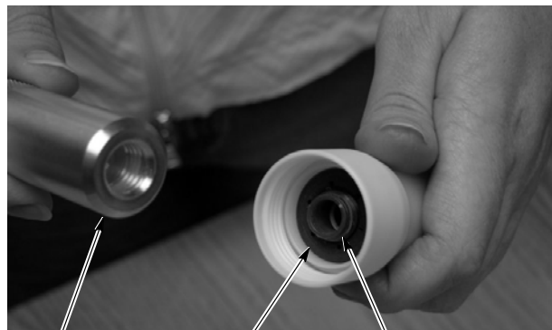
Figure 6 Nozzle Disassembly Step 1 (Shown with Nut Installed)
