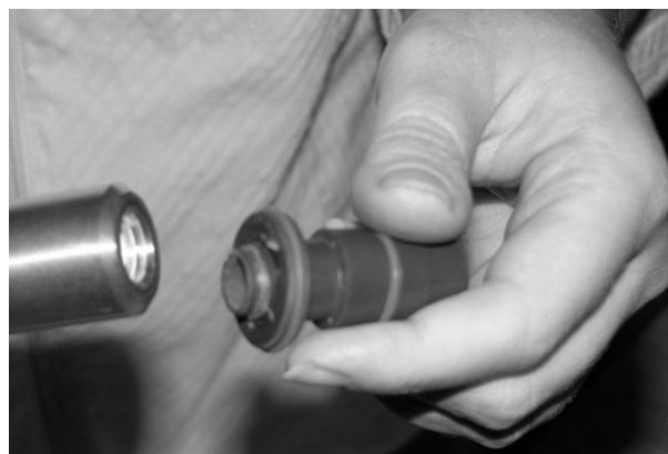
Figure 9 Nozzle Disassembly Step 3 (New Style Shown)
