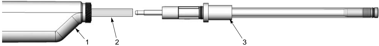
Figure 2 Connecting Powder Tubing to Lance Extension
