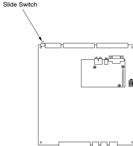
Figure 7 Power Switch Location
