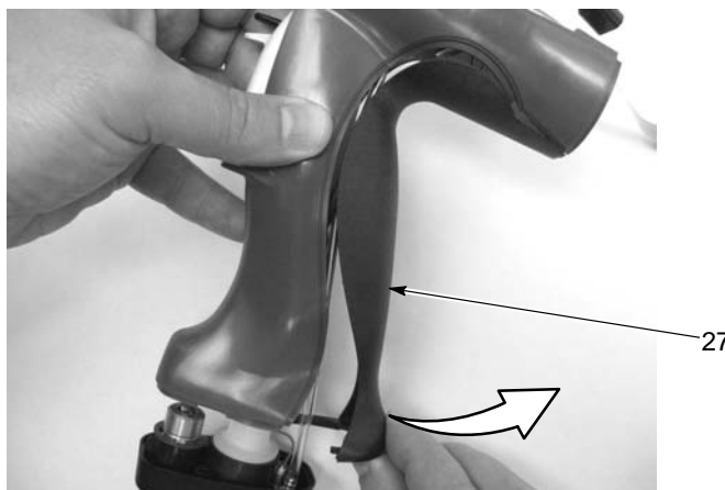
Figure 5-8 Removing the Ground Pad
