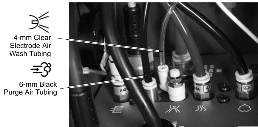
Figure 2-11 Connecting Air Tubing to the Power Unit
