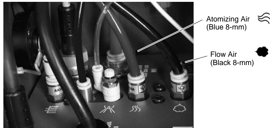
Figure 2-9 Flow and Atomizing Air Tubing Connections to Power Unit
