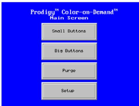
2. If starting with an empty system or if the system is filled with the wrong color, select a color and **START** a color change.
