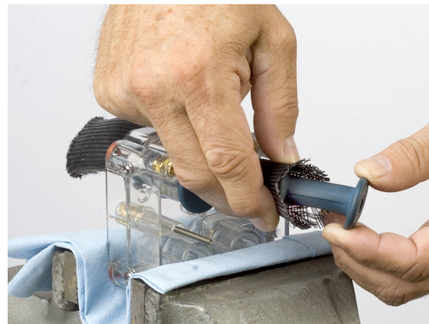
Figure 13 Inserting Pinch Valve into Insertion Tool
