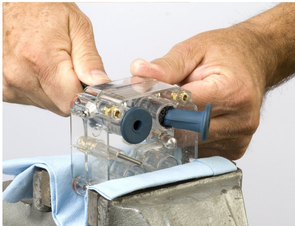
Figure 15 Pulling Pinch Valve into Valve Manifold
