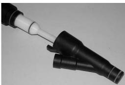
6. Unscrew the electrode assembly from the multiplier.
